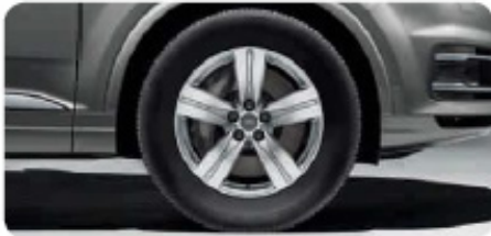
Forged aluminium wheels In 5-arm design size 8 J x 18 with 255/60 R 18 tyres 1
