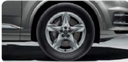
Cast aluminium wheels In 5-spoke star design size 8.5 J x 19 with 255/55 R 19 tyres 1
