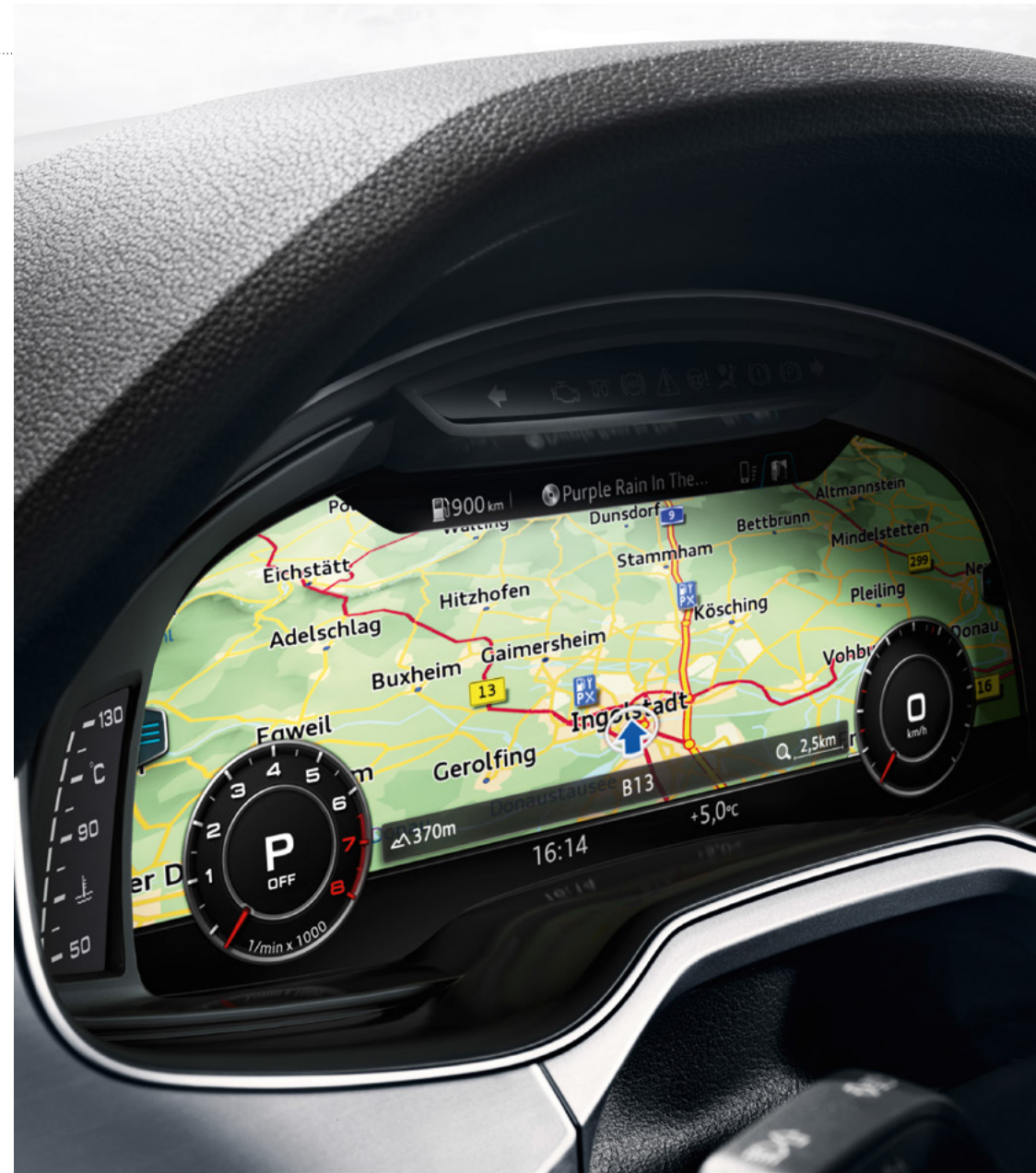
The Audi virtual cockpit is an innovative, fully digital instrument cluster embodying the progressivism of the Audi Q7 in the interior. The 12.3-inch LCD screen with a very detailed and brilliant resolution of 1,440 x 540 pixels replaces the classic instrument cockpit. Generally the Audi virtual cockpit offers two display
