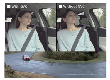
\* In-house passenger seat comparison of left-hand turn at 30 km/h (lateral acceleration of 0.4 G)
