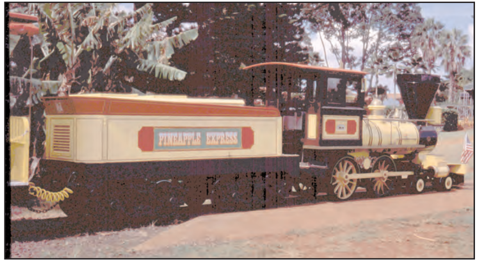
Above: Dole’s Pineapple Express alternates using its two locomotives, usually running each for about a month at a time. The bright yellow 4-4-0 was built at Stratford-on-Avon, England.
