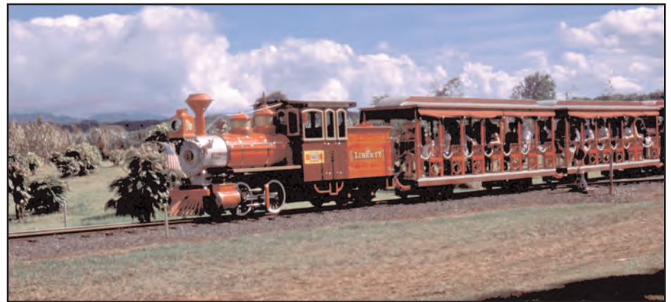
Below: This brilliant red two-foot gauge 0-4-4T at Dole Plantation is clearly designed after a 19th century Mason Bogie—until reality abruptly sets in as diesel exhaust billows out from under the cab.
