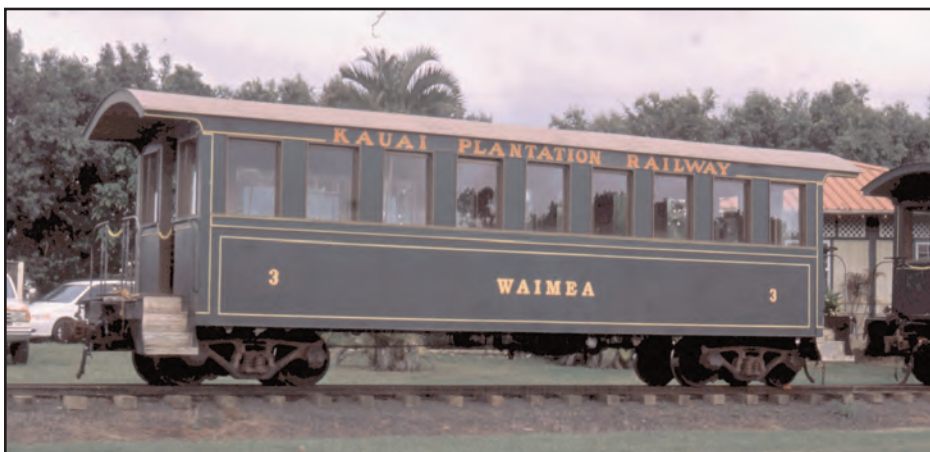
Below: Coach No. 3, Waimea, is typical of the four open-air passenger cars the Kauai Plantation Railway built up on 36-inch gauge ex-Hawaiian flatcars purchased from Alaska.
