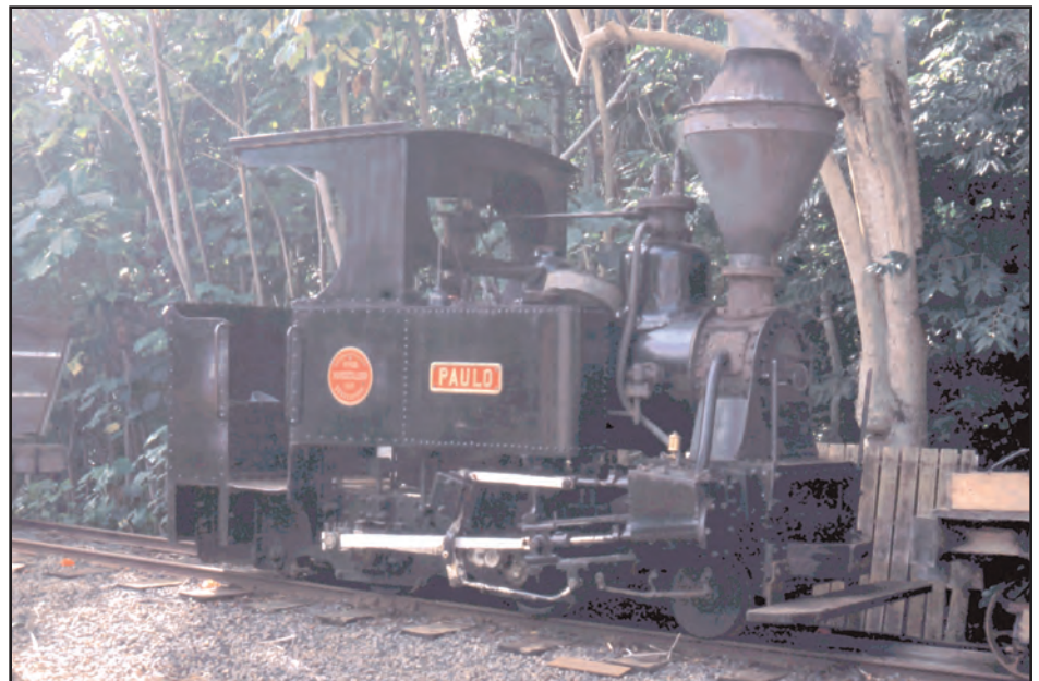
It’s a wood burner. What has to be one of the most historic locomotives in Hawai’i is the Paulo (Hohenzollern,Düsseldorf, Germany, 1887). The tiny 30-inch gauge 2-4-2T, often pulls—and pushes--the Grove Farm trains on the second Thursday of every month on the island of Kaua’i.
