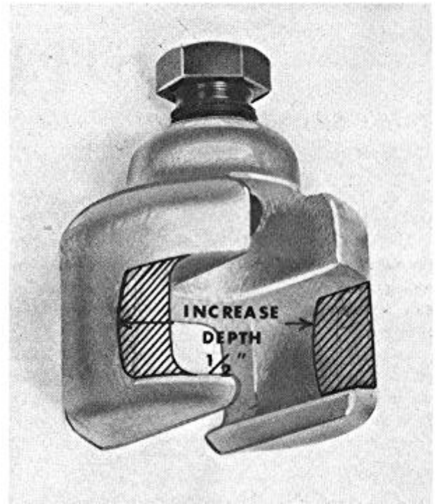
Figure 3—Revision to Tool J-1374 or J-5566
