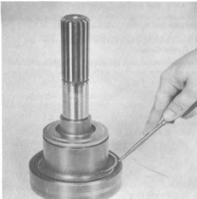
FIGURE 10— Remove the Snap Ring to Separate the Ring Gear from the Main Shaft
