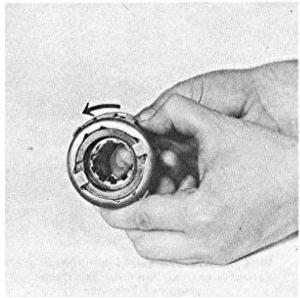
FIGURE 19—When You Twist the Cam Roller Retainer Counter-clockwise, the Two Springs Should Snap it Back Quickly
