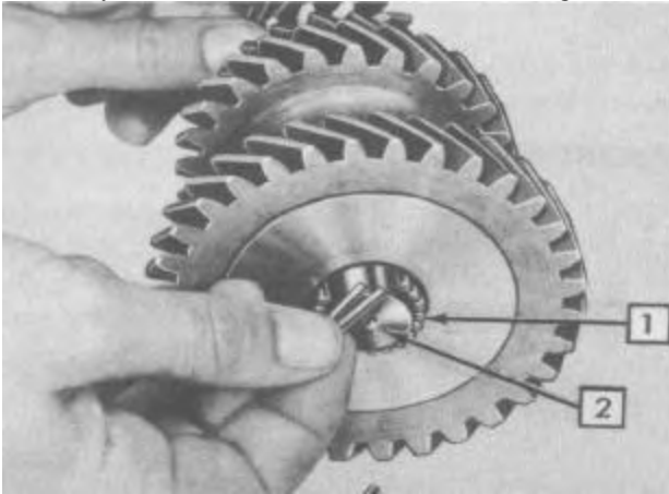
1. Needle Bearings 2. Dummy Shaft
