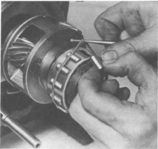
FIGURE 32—A Rubber Band Serves to Hold the Free Wheeling Rollers in Position until the Ring Gear and Main Shaft can be Installed
