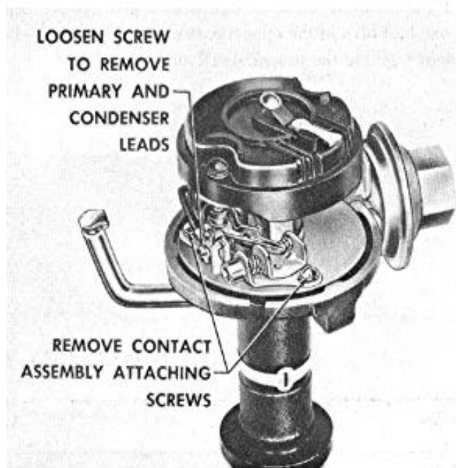
FIGURE 4—Removing Distributor Contact Set
