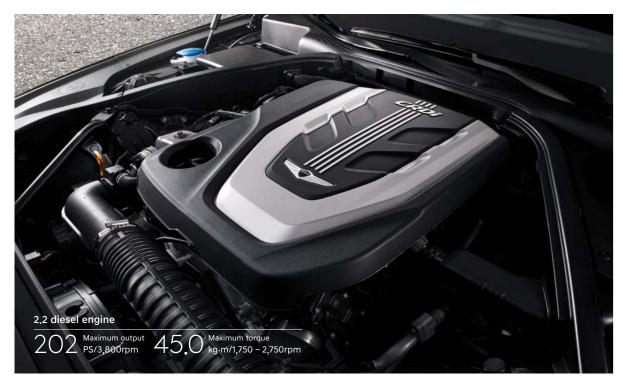
\*The diesel engine uses a selective catalytic reduction system that requires periodic replenishment of an aqueous urea solution.
