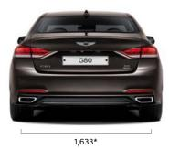
Units: mm. \*based on 245/40R19 tires in the front and 275/35R19 tires in the back
