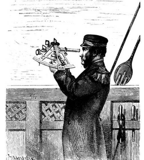
Sailor using a sextant The applications of Physical Forces, Guillemain, London, 1877, Library of the Musée d'histoire des sciences
