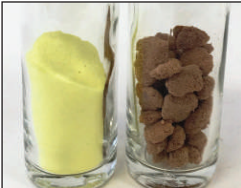
After absorbing mercury pollution, the rubber-like polymer changes color, indicating the job is done. More of the affordable polymer mixture can then be placed in the area to continue to process.
