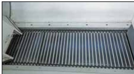
30.25" wide conveyor with 1/2" bars
