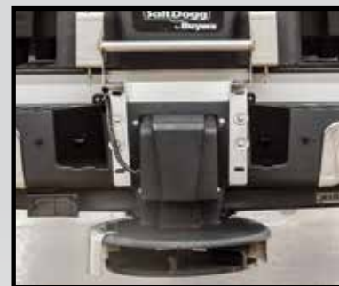
High flow swing away chute and large 14" spinner with 1/2 HP motor
