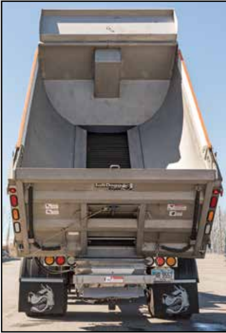
Unique, roll-formed sides and cross member-less design
