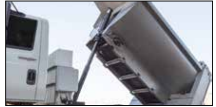
Mailhot® multi-stage, double-acting, nitrified cylinder, trunnion-mounted hoist
