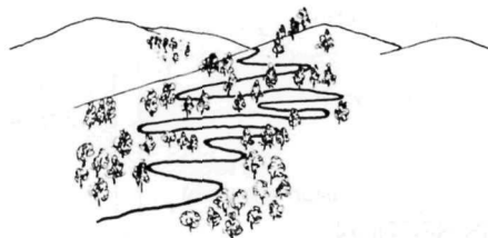
POOR PRACTICE — Landscape is damaged by short segments and numerous switchbacks. Repetition is monotonous to the user.
