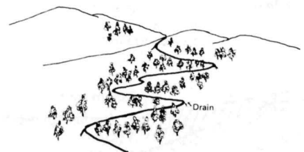
GOOD PRACTICE — Switchbacks are not intervisible. Use is made of natural topographic features, varying length of track segments between switchbacks for desirable variety and to prevent cross-cutting. Note also the drainage can be designed so the surface run-off collected does not affect the track segments below.
