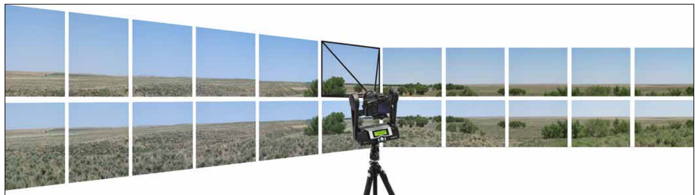
Figure 4.1.2-2. The GigaPan system takes a series of images that are stitched together using software to create a single panoramic image.
