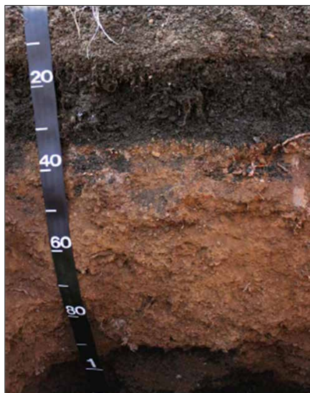
Figure 4.5.2-8. Buried soil at Lenox Crater. Scale is in centimeters. The upper 10 cm are light brown as they contain loess deposited since the eruption of Sunset Crater. At ~ 35 cm is the contact between the black Sunset Crater tephra and the brown buried pre-eruptive soil, a result of the accumulation of loess, aerosolic silt and clay deposited on the ground surface. Photo Credit: © USDA 2014.
