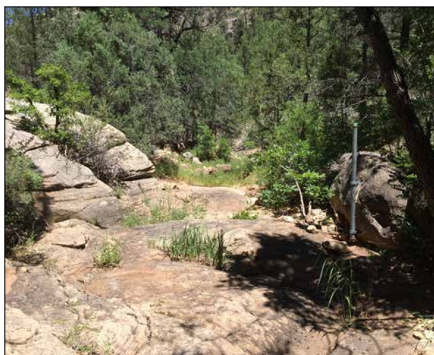
Figure 4.5.2-2. Photo of the recording stage gage at Cherry Creek. Photo Credit: © Steve Monroe, SCPN Partner.
