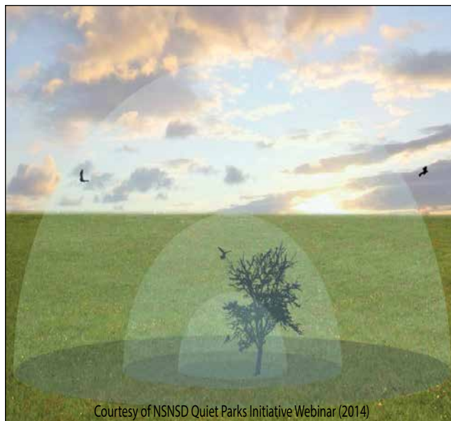
Figure 4.3.1-2. A 6 dB reduction in background noise level would produce a 4x increase in listening area. Figure Credit: © Ted E. Dunn.
