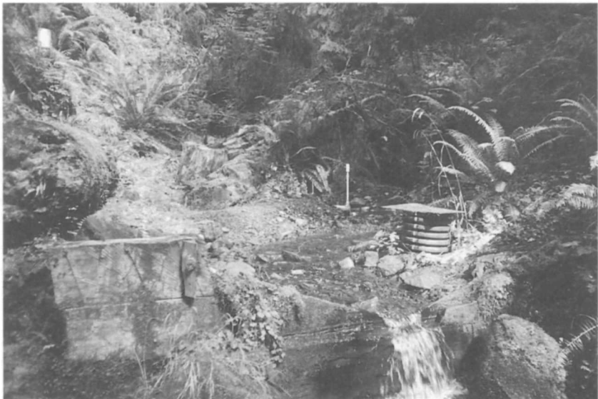
Figure 18. The 3:1 V-notch weir at West Twin Creek, showing the stilling well in the foreground and the proportional flow sampler in the background
