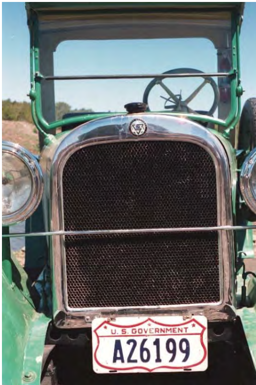
The Albuquerque shop put Federal Shield plates on the 1925 DB. Note the honeycomb radiator.
