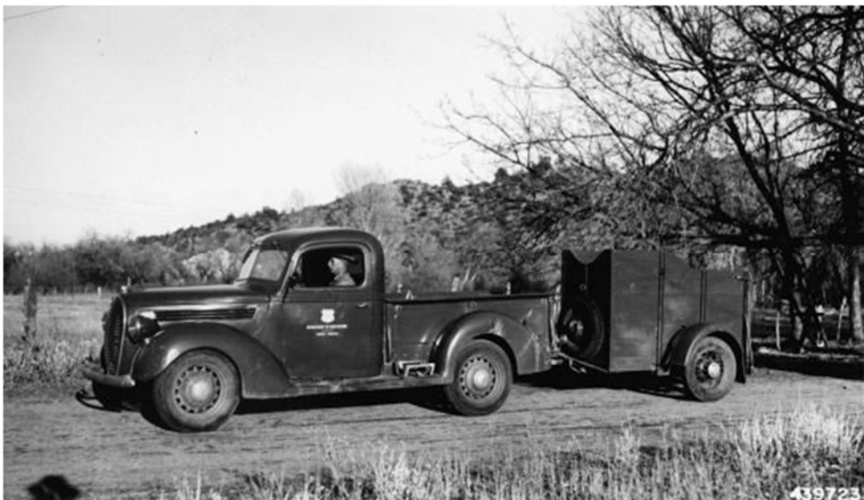
The FS vehicle in this 1946 photo is of a Tonto NF 1939 Ford pickup with horse trailer. The markings on this vehicle consist of the three-star, red white and blue, 4 1/8-inch-tall "U.S. Government" "For Official Use Only" aluminum shield above a decal that reads "Department of Agriculture" ----- "Forest Service." The color was Dark Green. The door markings changed from the type 2 FS shield. This truck has no vehicle number on the door.
