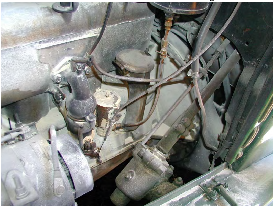
Fire extinguisher dust on the engine after the 2007 fire.
