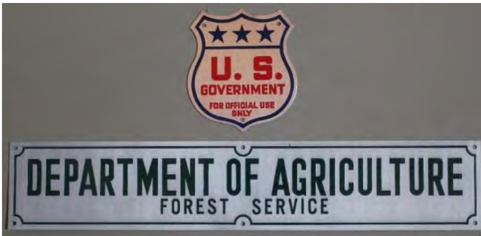
Aluminum FS vehicle door markers were used from about 1956 to mid-1960's on some forests. These markings had to be screwed or riveted to the door. The U. S. Government shield is sometimes miss identified in photos of FS vehicles as being a FS shield.
