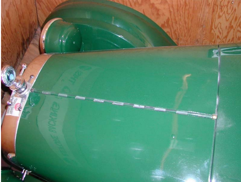
The outside of the hood did not show much fire damage.
