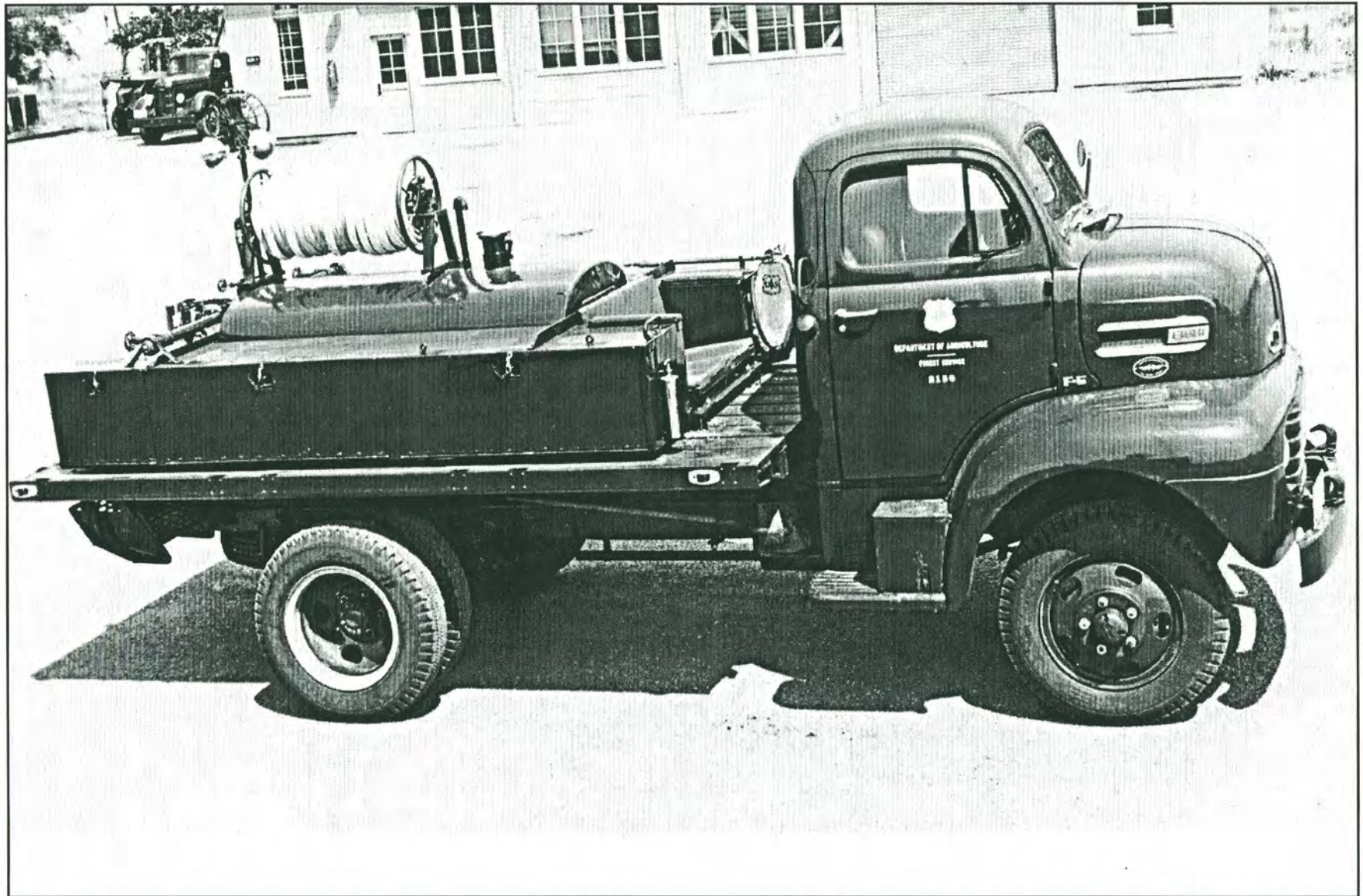
FS #2150, 1948 Ford COE with "Marmon Herrington" all wheel drive conversion. This rig is a Model 48 slip-on unit with a Model 120 Edwards pump and pump motor on the rear. Tank capacity is 250 gallons. Photo was taken at the Stanislaus National Forest Equipment Shop. The Model 49 soon followed which moved the hose reel crosswise on the rear with the pump and motor.
