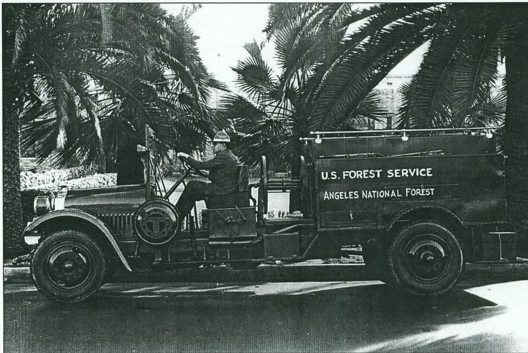
One of the Angeles National Forest's first tankers. Truck chassis is a heavy duty "White Truck," maybe late '20s or early '30s. The tanker does not appear to be outfitted yet. Photo was probably taken at time of delivery. The spare tire must have been an option back then.
