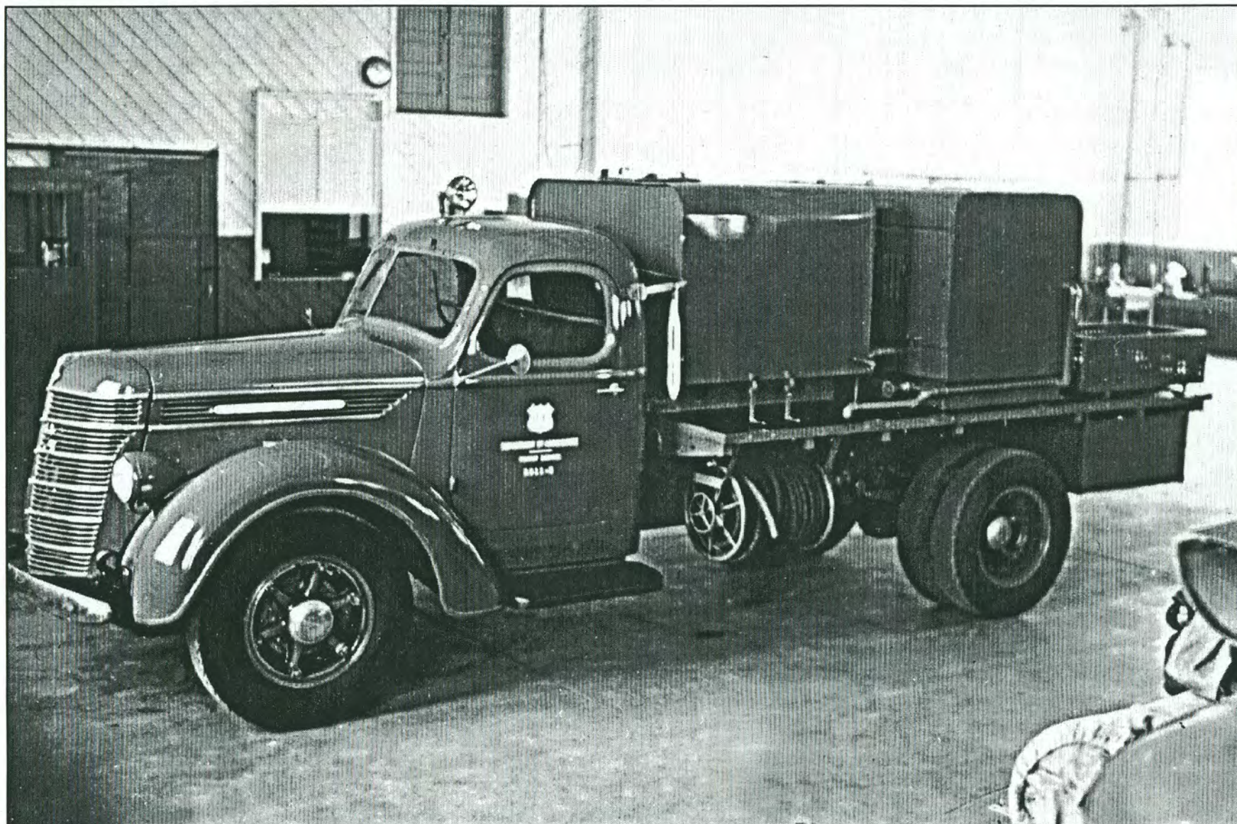
FS #1811-G, 1944 International Truck. This is a flatbed tanker with a slip-on unit built at the Salinas Depot for "building protection." The pump is a high pressure Royal Bean 35 plunger type. Tanks are 400 gallons each, one water and one foam. Truck appears to be red instead of dark green.
