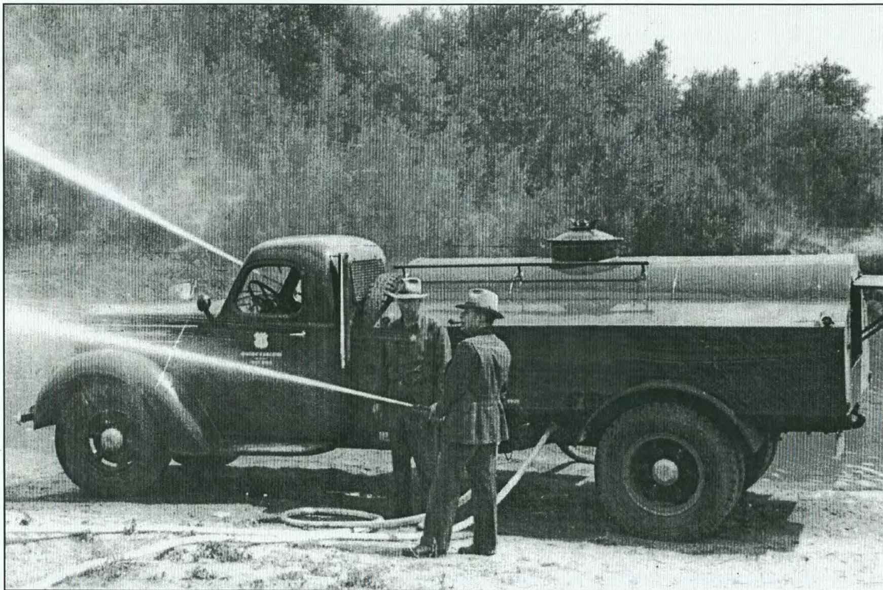
FS #2526. 1944 International Forest Service tanker. This unit has a PTO pump and a large capacity tank. Photo taken at pump testing on the Calvares River, 7/15/44.
