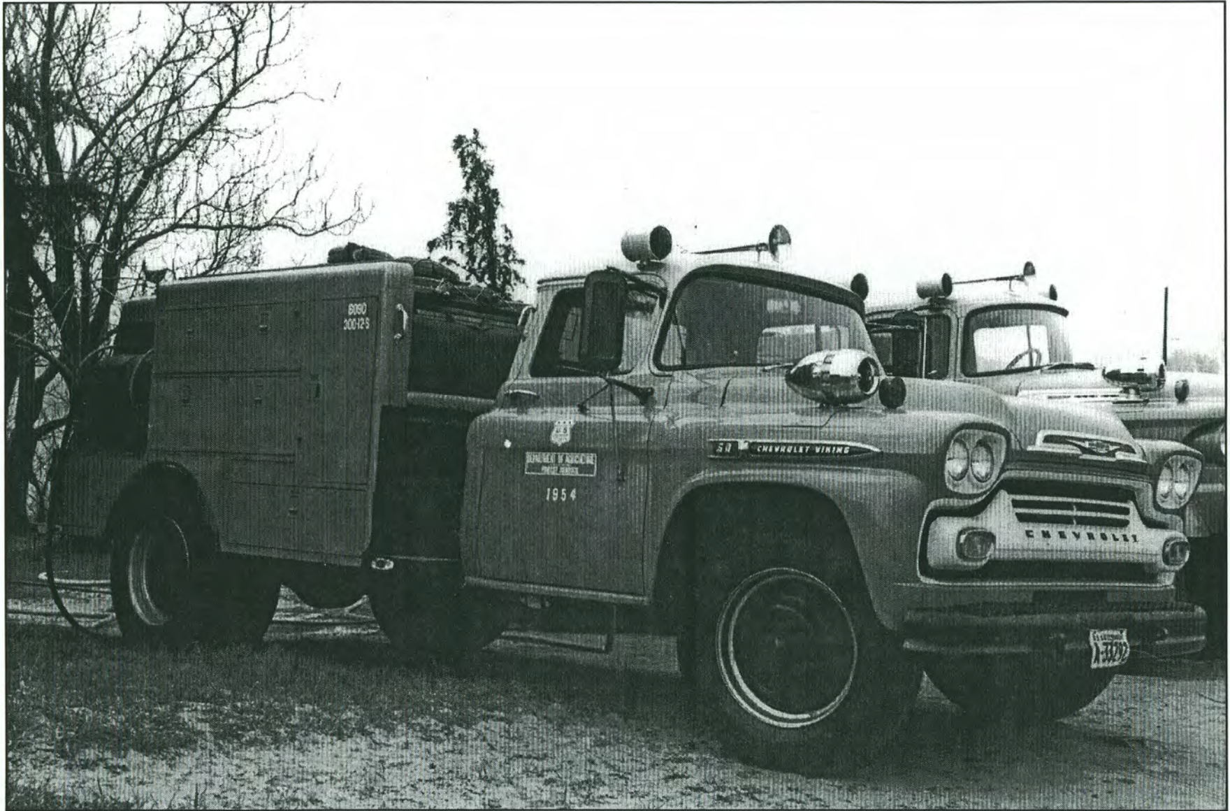
FS #1954, a 1959 Chevrolet Model 56, San Bernardino National Forest. Forest Service went to the light green (Safety Green) and grey cab tops around 1955 or 1956. The Model 56 was a popular model which saw service for a long time. The Model 56 came on various chassis, International, Dodge, Ford, and Chevy. Photo was taken during a structure fire training exercise on the San Bernardino National Forest.
