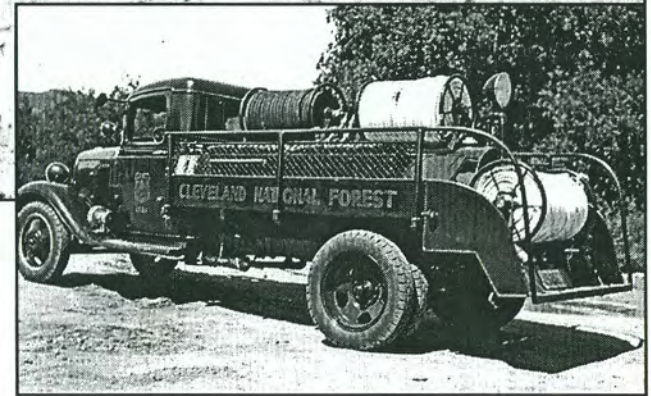
FS # 1134 is a 1934 Chevrolet Forest Service tanker with a 2" Viking PTO pump and 200 gallon tank. This unit saw service on the Cleveland National Forest. This model carried 2 live reels on top and the rear reel was not charged. Writing on the back of the photo said that it carried tools and a 10 man crew. The Cleveland also had similar tankers on a '37 Chevy FS #1969 and a '33 International FS # unknown.
