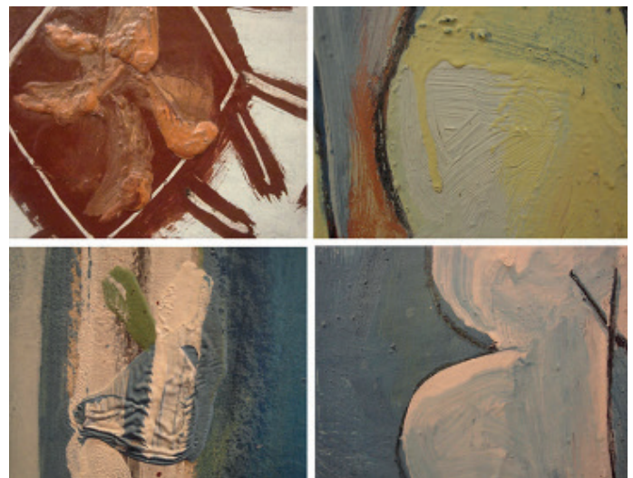
1. Selected examples of surface characteristics typically associated with enamel paints, as captured on the surfaces of the Antibes paintings. From top left, clockwise: fluidity of paint; drips; marbling and incorporation of dried bits of paints; wrinkling. Details taken from, top left: Nature morte aux volets noirs ; top and bottom right: La Joie de Vivre ; bottom left: Ulysse et les sirènes
