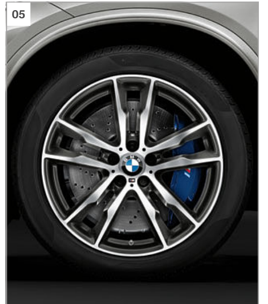
[05] 20" M light alloy wheels Double-spoke style 611 M, gloss-lathed with mixed tyres, front size 10 J x 20 with 285/40 R 20 tyres, rear 11.5 J x 20 with 325/35 R 20 tyres.
