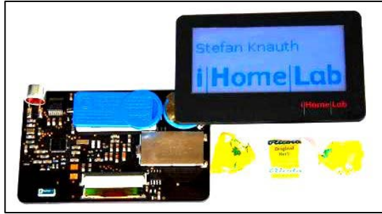
Fig. 3. Name badge with IEEE802.15.4 radio transceiver, ultrasound transmitter and cholesteric LCD
