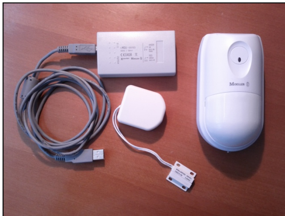
Figure 1. Eaton Xcomfort sensors and gateway
