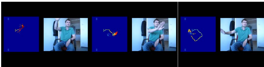
Figure 1. Sequence of still images of an example of raw hand tracking data from the UCOS2 sensor (left pane) and synchronous video (right pane) for a person performing a “circle” gesture with his right arm.
