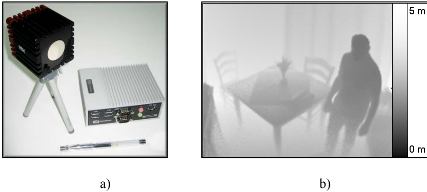
Figure 1. a) Hardware platform overview. b) A typical range image with the related gray scale distance. It is also apparent, as the person's identity cannot be revealed from range images.
