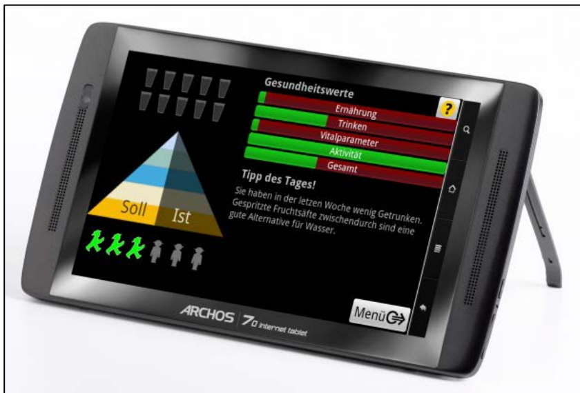
Figure 1: An example of a lifestyle management application for elderly people detecting eating and drinking habits as well as activity and providing direct feedback by changing colours of symbols (drinking glasses) and on the collected data via “personal advice”. The application is ANDROID based and runs on a tablet PC.
