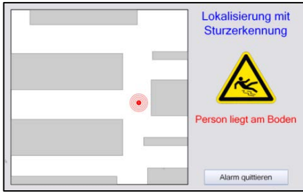
Fig. 6. Fall detection application: The name badges transmit acceleration sensor data to the system. In the case of a fall, an alert is generated, indicating the location of the incident
