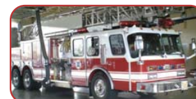
1999 E-One Hurricane 100' Quint Cummins Diesel, Allison Automatic Hale 1500 GPM Pump 400 Gallon Poly Tank 100' Akron Monitor at Tip Call for Pricing
