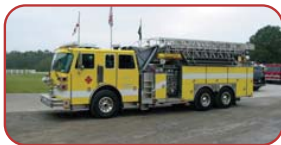
1993 Sutphen 75' Quint Detroit Diesel, Allison Automatic Hale 1500 GPM Pump 500 Gallon Booster Tank Akron In-Line Foam Eductor $199,000
