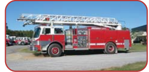
1985 Hahn/LTI 75' Quint Detroit Diesel, Allison Automatic Waterous 1500 GPM Pump 400 Gallon Tank Quartz Scene Lights $99,000
