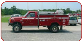
1990 Marko 4x4 Quick Attack Int'l Diesel, Ford Automatic 90 GPM Gasoline Powered Pump 200 Gallon Polypropylene Tank Call for Pricing
