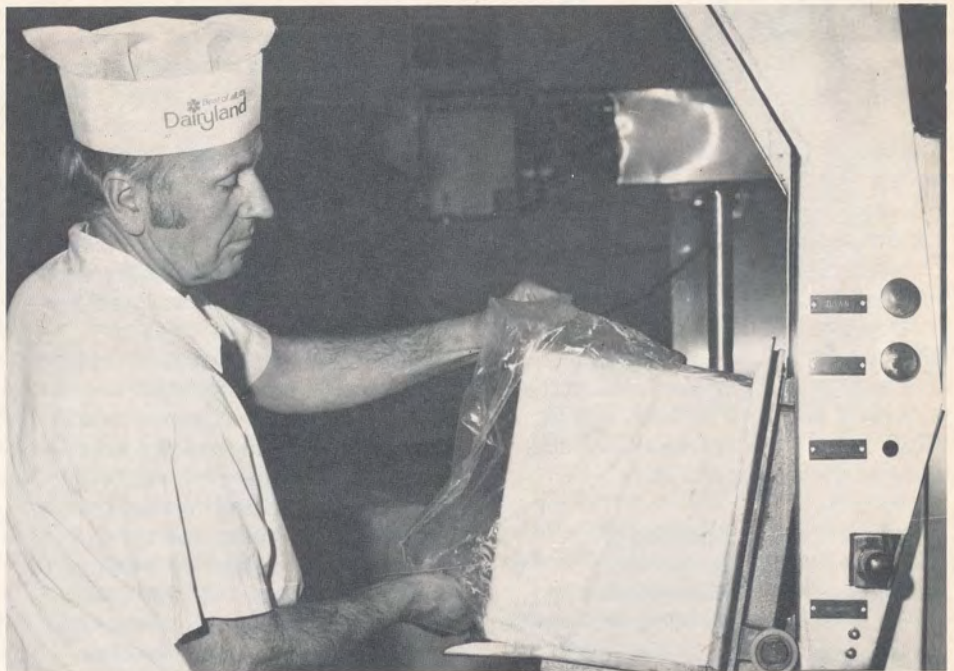
Butter will be lifted to a chute at top of reworker. Operator is Henry Dyck.
