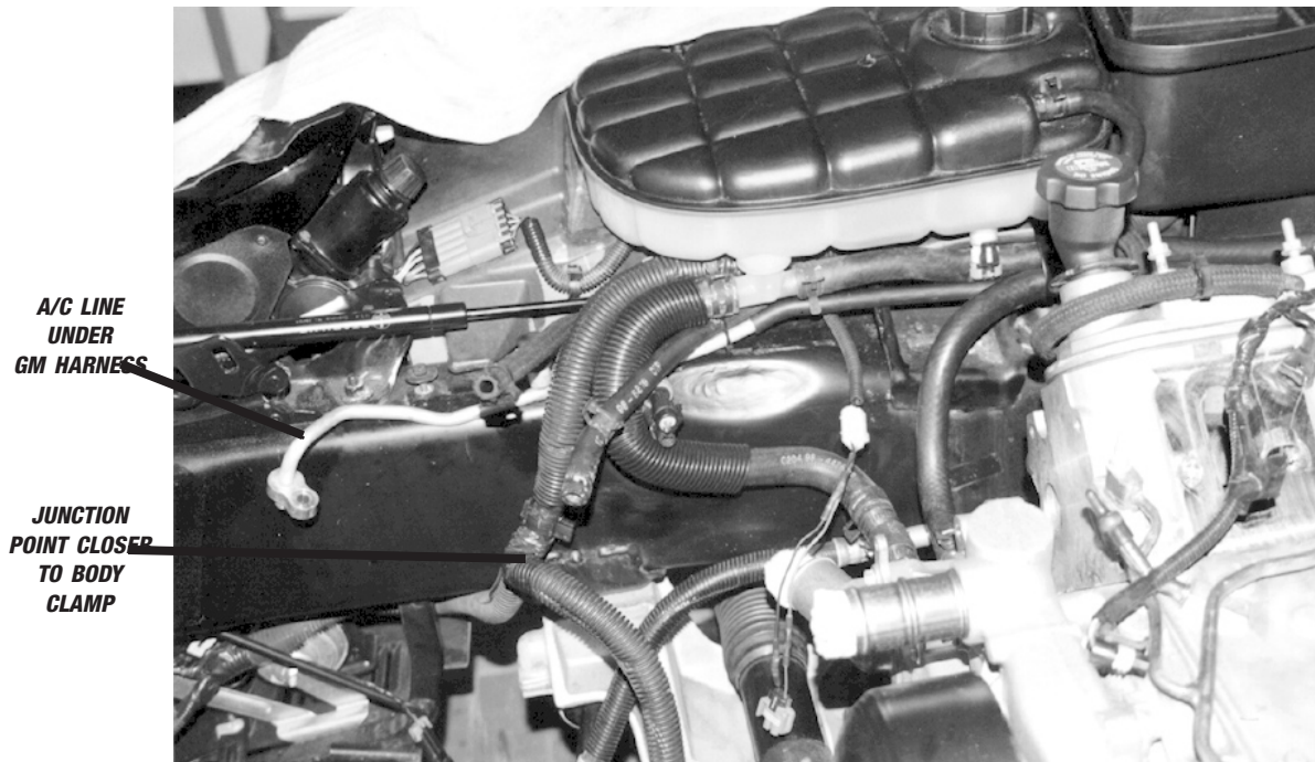
— FIGURE 6.17 — THIS IS HOW THE A/C LINE & GM HARNESS SHOULD LOOK WHEN COMPLETED
