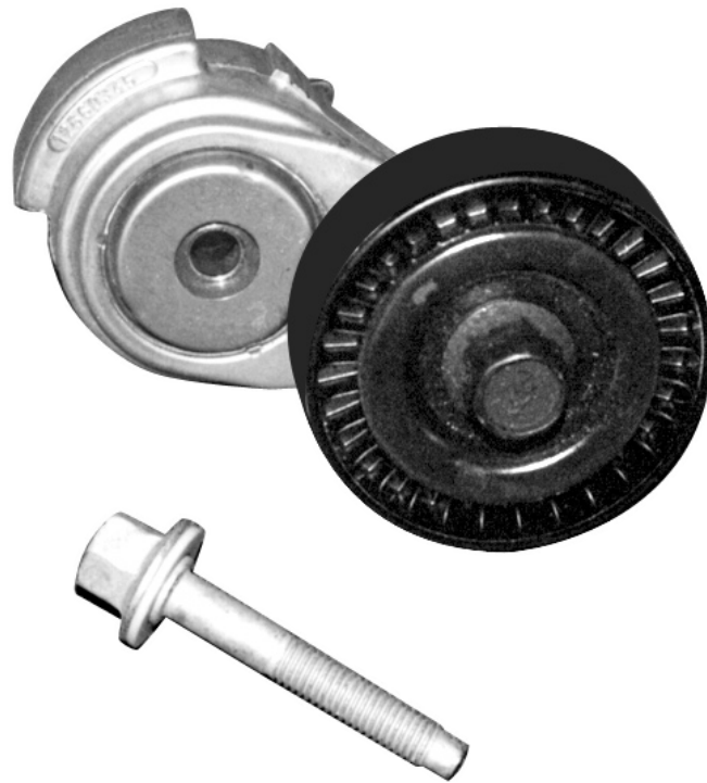
— FIGURE 1.66 — GM A/C BELT TENSIONER & BOLT USED TO FASTEN TO ENGINE.
