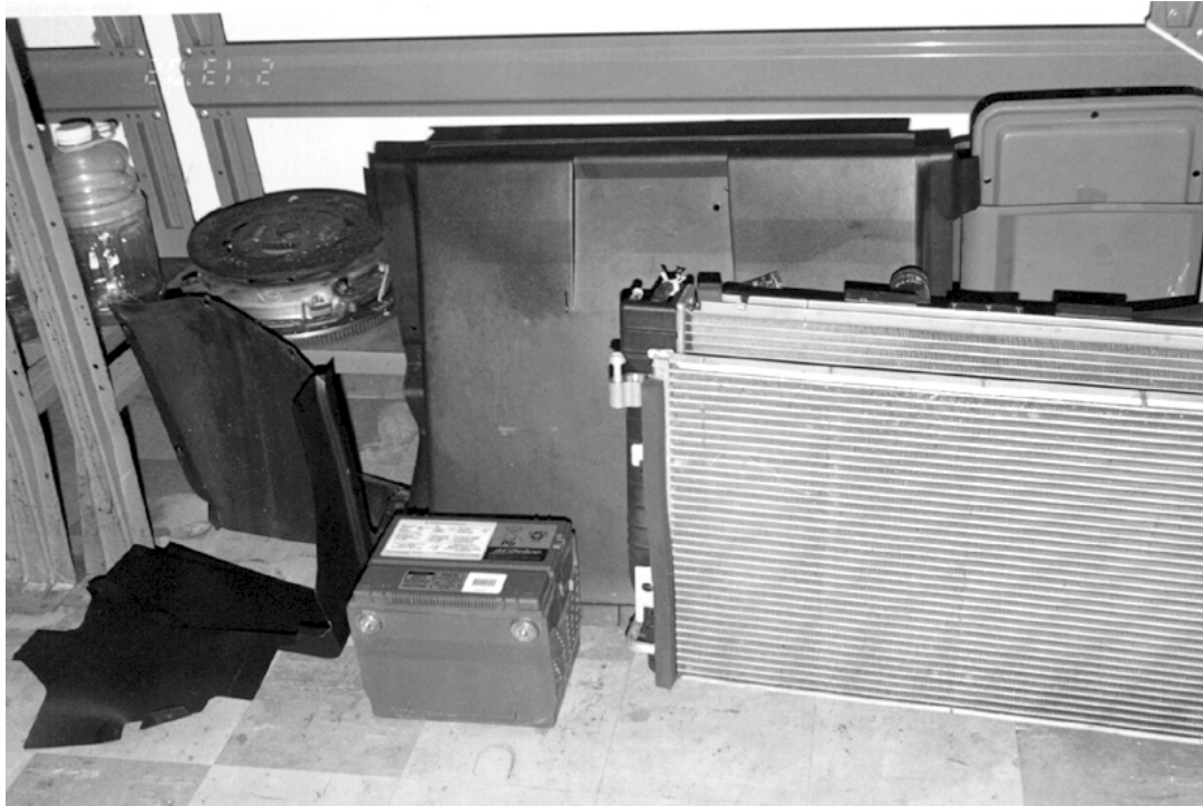
— FIGURE 1.38 — VIEW RADIATOR – A/C CONDENSER SHROUD ASSEMBLY AFTER REMOVAL FROM ENGINE COMPARTMENT.
