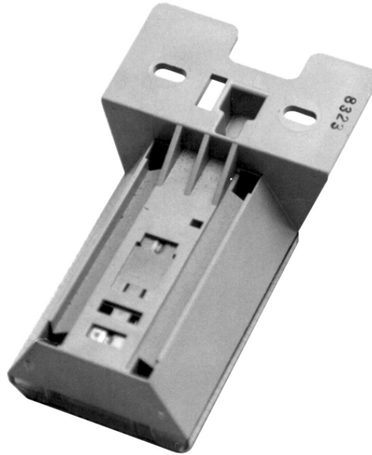
— FIGURE 17.1 — UNDERHOOD LAMP ASSEMBLY PRIOR TO MODIFICATION
