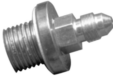
— FIGURE 3.4 — MODIFIED GM OIL PLUG WITH #3 AN ADAPTOR
