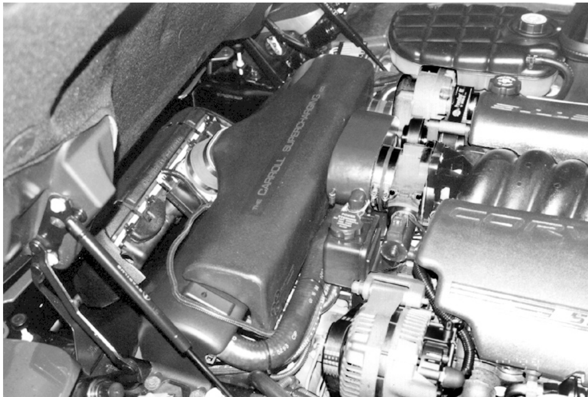
1999 C5-LS1 CORVETTE • STAGE I SUPERCHARGING SYSTEM • NOTE STOCK GM AIR FILTER
