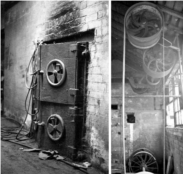
The germination floor, furnace of the 1890 kiln and belt drives. At the bottom right are the maltings buildings in 2018..
