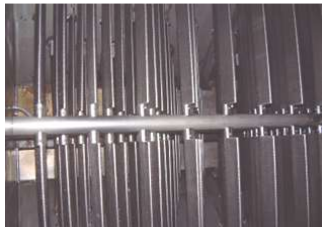
The internal run off pipes and the attached perforated lobes
