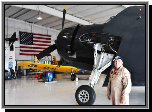
The finished product, with a team member next to the massive left gear. The wings fold much like the Hellcat's wings. The TBM is a large airplane, and needs constant attention by the pilot to trim controls to fly.
