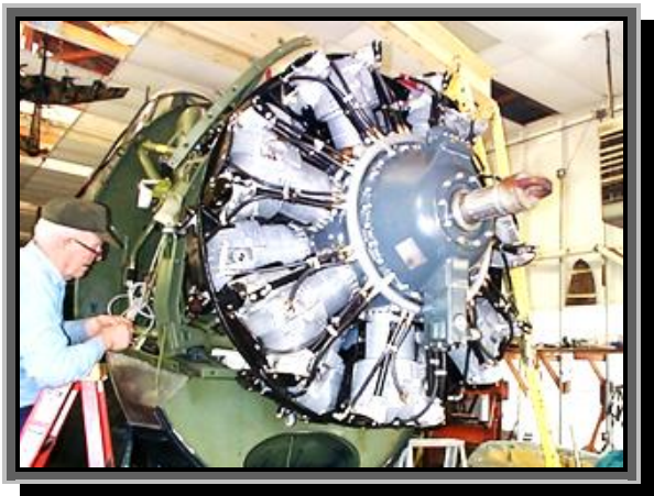
The TBM's engine – 1,900 hp Wright R-2600-20.
