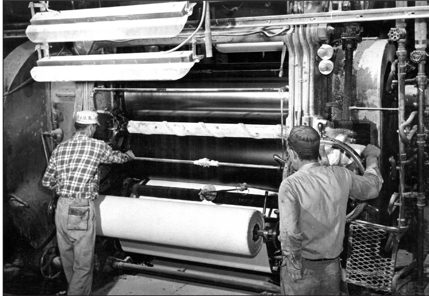
"Few photos exist of the multistep process of manufacturing Haartz cloth years ago. Although this image dates from the early 1950s, it shows one step that was also normal procedure prior to WW2 in the Haartz-Mason plant. This machine is a rubber calender. Rubber stock, fed from above into a three-roll stack, was milled down to a consistent film thickness and pressed onto cloth at the bottom roll." Photo from Haartz Corporation Archives
