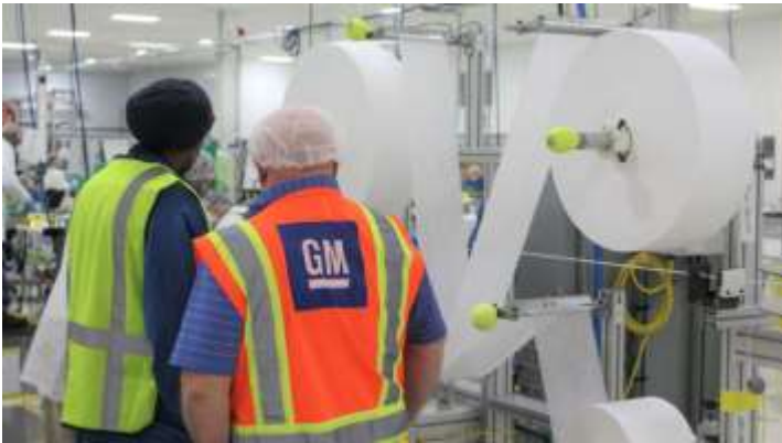
General Motors workers at its face mask production at a plant in Warren, Michigan works on a machine at the beginning of the process that ultrasonically welds three layers of material into one, crimps the front of the masks and inserts the metal line, or nose wire, in the mask.
