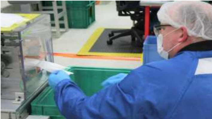
Face masks are cut by a machine and spit out faster than an ATM machine dispensing bills. The machine ultrasonic welds three layers of the material into one, crimps the front of the masks and inserts the metal line, or nose wire, in the mask.
