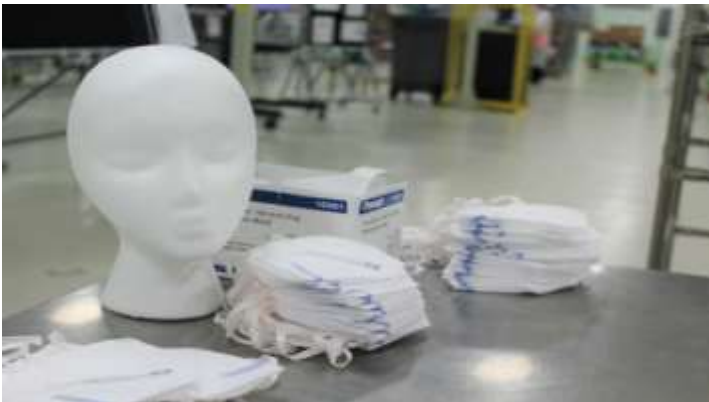
General Motors is beginning to produce N95 masks at a former transmission plant outside Detroit. The manikin head is being used to test the fit of the masks prior to distribution.
