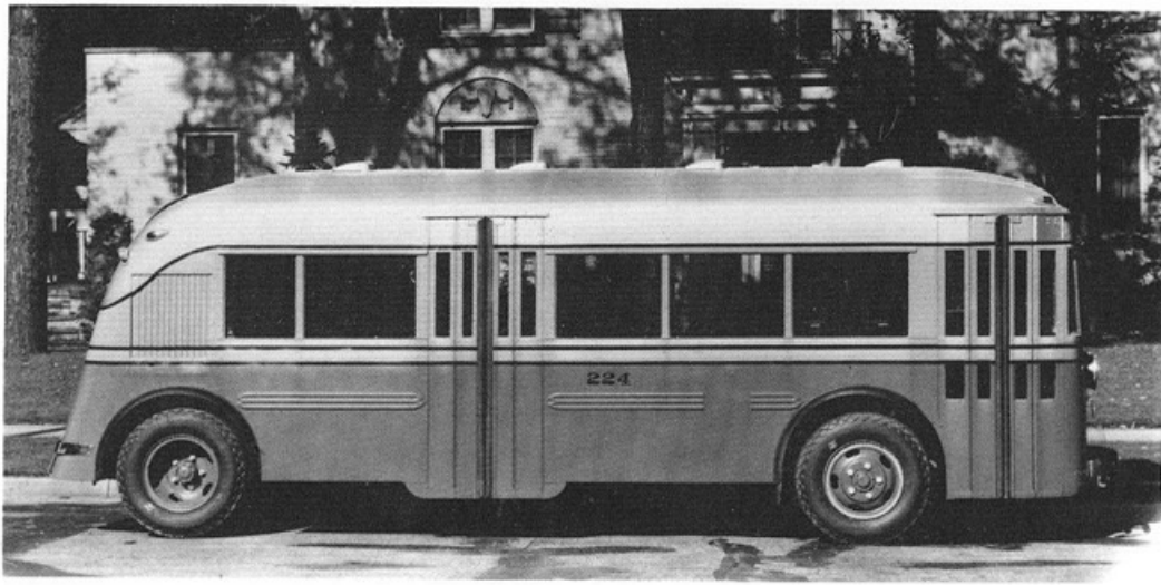
Purchased for the conversion of the Leonard & West Mound car line, which took place on December 29, 1935, were eight Twin Coach 23-R's, the first Columbus buses with rear engines. —Twin Coach
