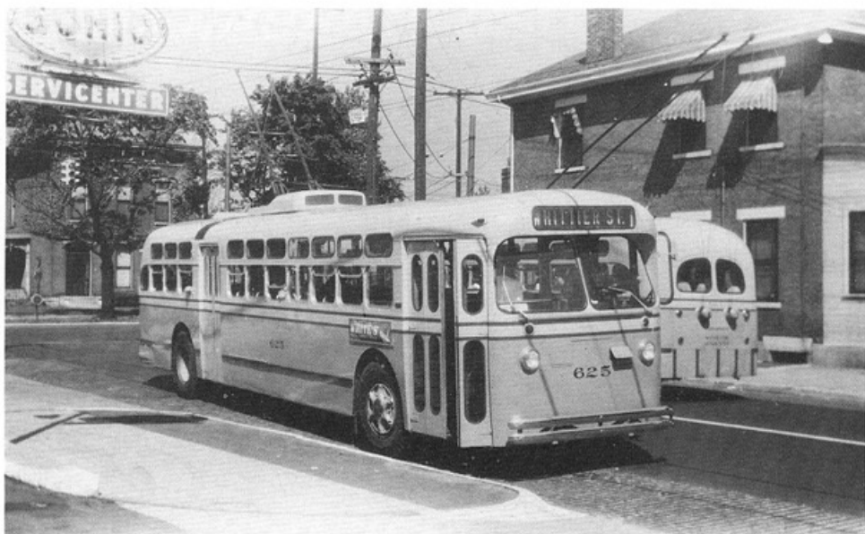
The 600's took over on the High Street lines as they were delivered, releasing smaller 500's to convert Main, Neil, and Parsons to trolley-coach in September 1948. The picture shows that the front doors of the Columbus Marmons could be operated individually. —Robert S. Crockett
