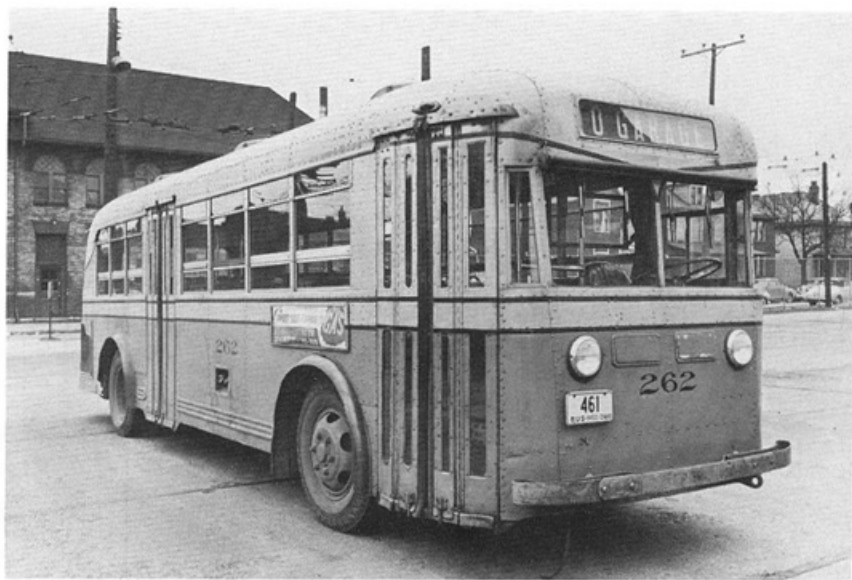
Two types of prewar Twins: 262 was a 31-R built in 1938, and 270 was a 35-G of 1941. In Twin Coach nomenclature "R" meant rear engine and "G" meant gravity suspension, a torsion bar arrangement used in place of leaf springs.
