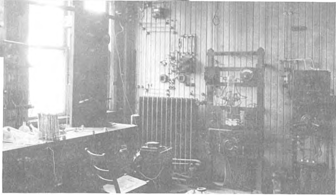
Steinmetz's physical laboratory, with an early model of his mercury arc rectifier mounted on the wall.
