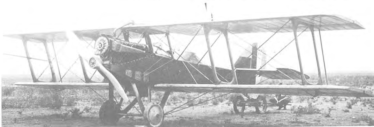
LePere biplane powered by Liberty engine equipped with Moss turbine driven supercharger.
