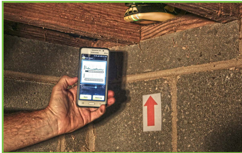
Termatrac's three-in-one sensor with radar, thermal and moisture detection abilities communicates through a smart phone app. Pest inspectors can print and record data to show homeowners their findings.
