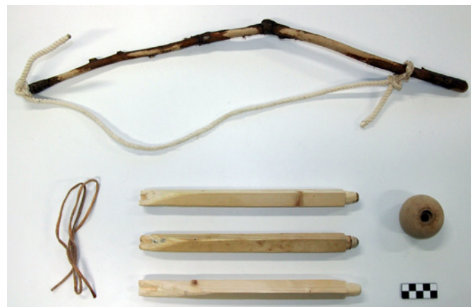
Perforation equipment used in the experiment : components of a bow drill.
