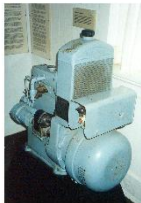
Kohler Electric Generator
