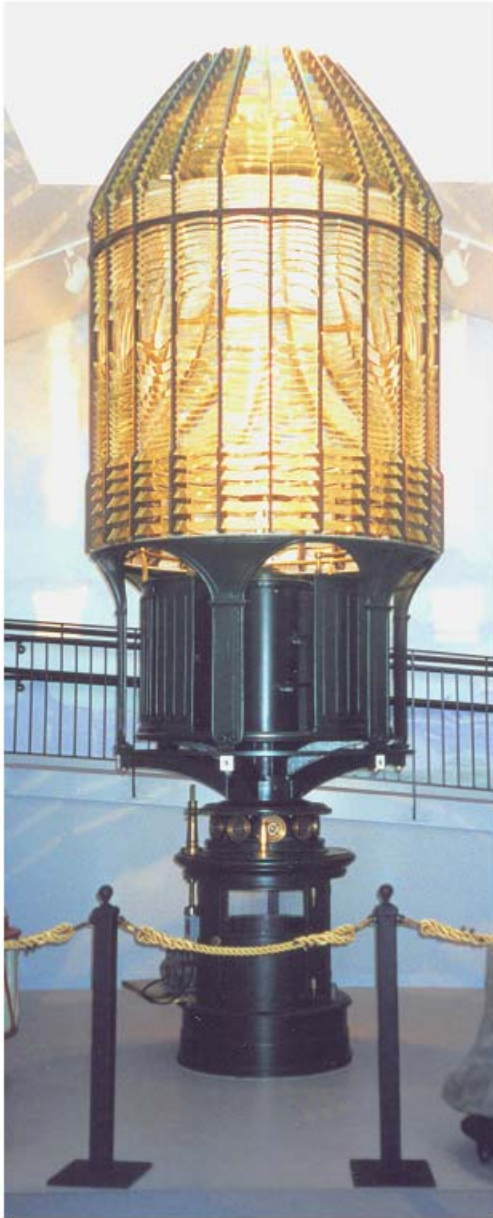
First Order Fresnel Lens Made in France - Removed from Destruction Island Lighthouse and placed on display at Westport Maritime Museum, Westport, Washington
