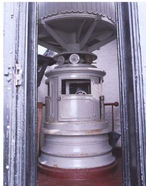
Lens Rotating Mechanism – Cape Hatteras Light
