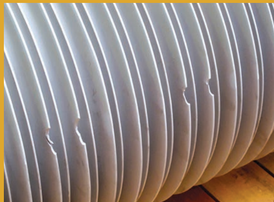
Shed damage from mishandling.
