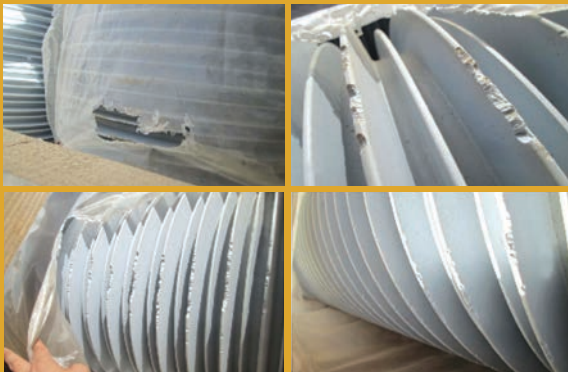
Bushings with damaged composite housings received by utility in Middle East.
