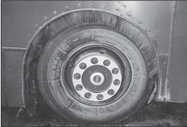
Swedish Teastrainer? The "6th Profile" front embellisher, seen here as fitted to Preston Bus AN68D/2R in maroon livery.
