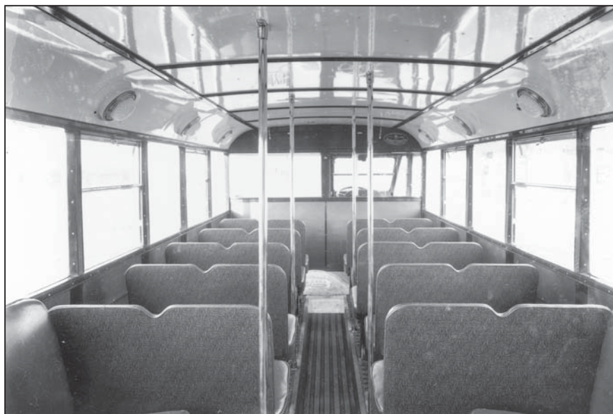
This view illustrates the interior of a highbridge TD1. Seats like those in this picture were taken from withdrawn Liverpool Titans and fitted into AEC Regents similar to the one seen above, as there was an acute shortage of seat rails at the time (1946-7).
