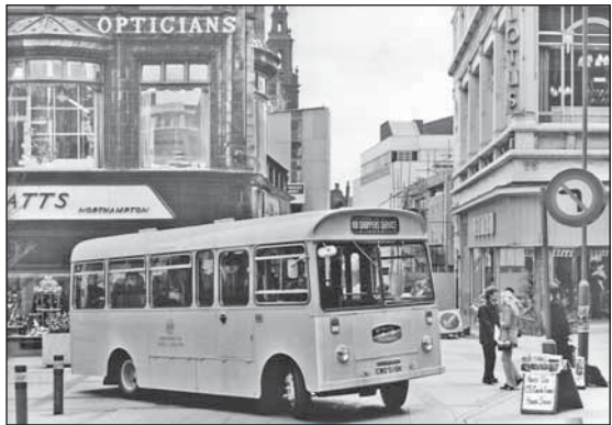
CWO 519K was one of the two Crompton-Leylands, bodied by Willowbrook, and badged as Morrison Electricar.
