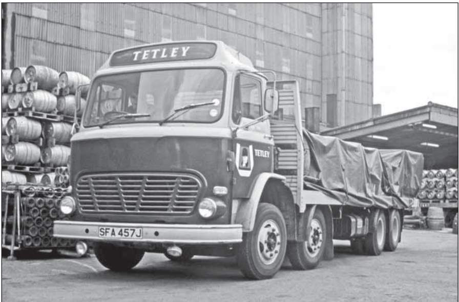
Breweries often required special vehicle designs to suit their loads and this 1971 Laird is no exception, probably having been converted from a standard chassis by a specialist company, using standard axles and other parts. It is seen in Leeds in May 1973.
