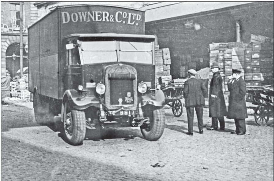
Photographed in March 1932, the radiator blind suggests that Spring had not yet arrived! This Buffalo TSQ3, owned by Downer & Co, was delivered to L. A. Evans of Southampton in January 1931, registered TR 9917, with chassis no.653. (BCVMT L010970)
