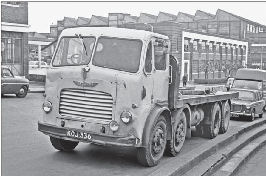
After twelve years of hard work, this 1953 “mouth-organ” cabbed Octopus 22.0 was beginning to show signs of a hard life when it was photographed in Luton in May 1965. The rust stains around the radiator filler suggest that overheating has occurred at some time.
