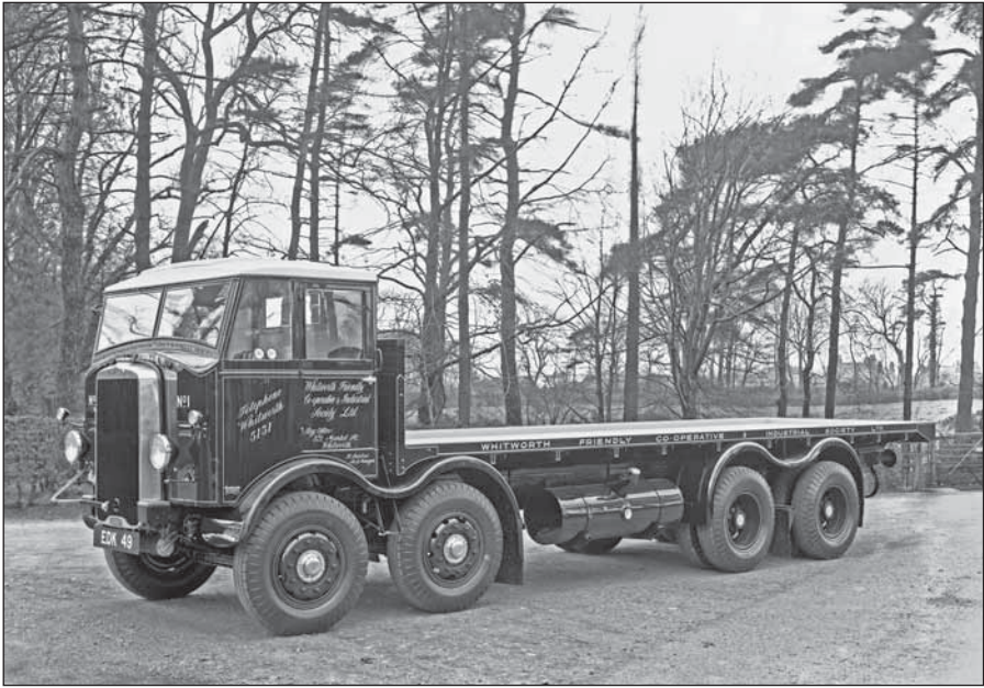
The 1939 sales brochure for the Leyland 8.6 litre oil engine quoted the Simms fuel pump for goods models such as this Rochdale registered Octopus TEW15D, chassis 303001, supplied to the Whitworth Friendly Co-operative Industrial Society in April 1939.
