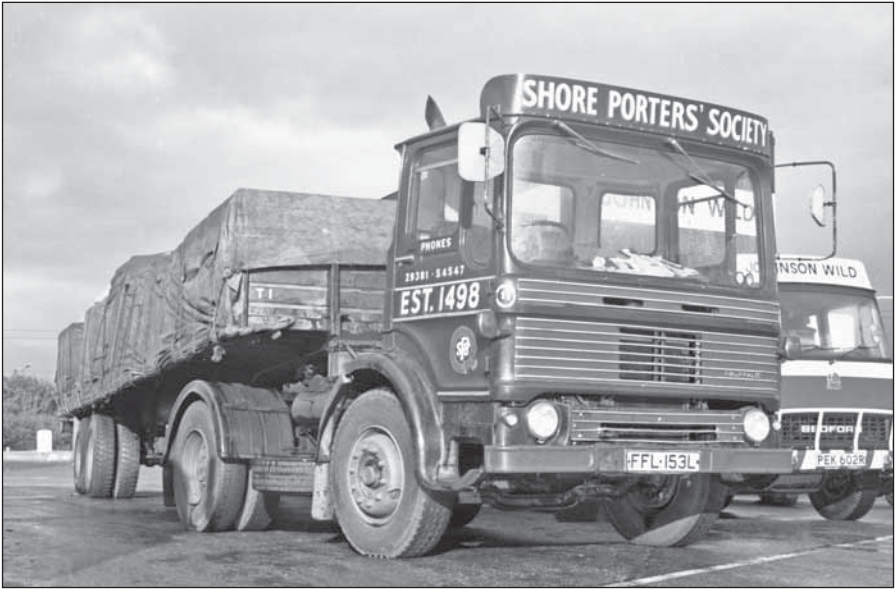
A 1973 Buffalo, photographed at the Services on the M1 at Toddington in August 1979, with a sheeted load on the semi-trailer. It was powered by the turbocharged version of the 500 engine, driving through a fuller gearbox to a Leyland hub reduction axle.
