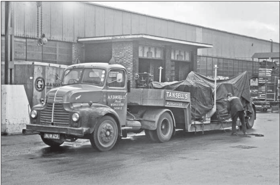
An unusual Comet artic, NUW 129 - it would be interesting to know what this 1953 Comet ECO2/5R was delivering to the Vauxhall Motors factory in February 1966. Judging by the deflection of the bed of the single axle trailer it looks to be heavy! Originally built for Shell Mex & BP, it has a front mounted silencer to comply with Petroleum Regulations. (Peter J Davies)
