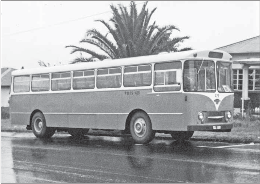
POTS 429, TDL 11901, was a Worldmaster ERT2/1, chassis 802007 (line no.1905), new in 1970 with Crown B64 (3+2 seating) + 24 standing body, in Edenvale.
