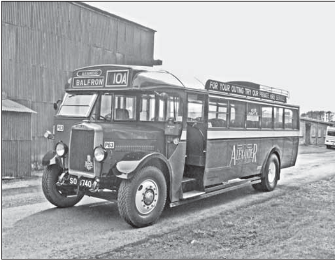
SO3740, a 1929 Leyland Tiger TS2, 60381, rebodied with 1934 Alexander B32F body when fitted with an 8.6 oil engine. Found as a static caravan at Newmill, Banffshire in 1974 and restored to 1934 condition.
