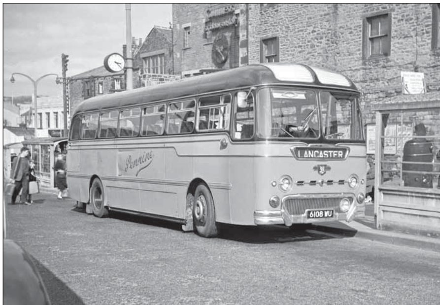
An attractive Duple-bodied Leyland Tiger Cub PSUC1/2 of early 1960 (chassis 596827, line no 952) operated by Pennine Motor Services, Gargrave, the well known and much appreciated operator that unfortunately has ceased operations in May this year.
