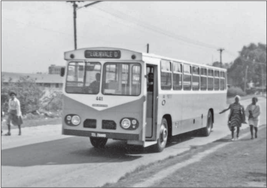
POTS 441, TDL 20085, a later Worldmaster, model ERT2A/1, chassis 7103870 (line no.2007), new in 1971 with Crown B70 (3+2 seating) + 23 standing body.
