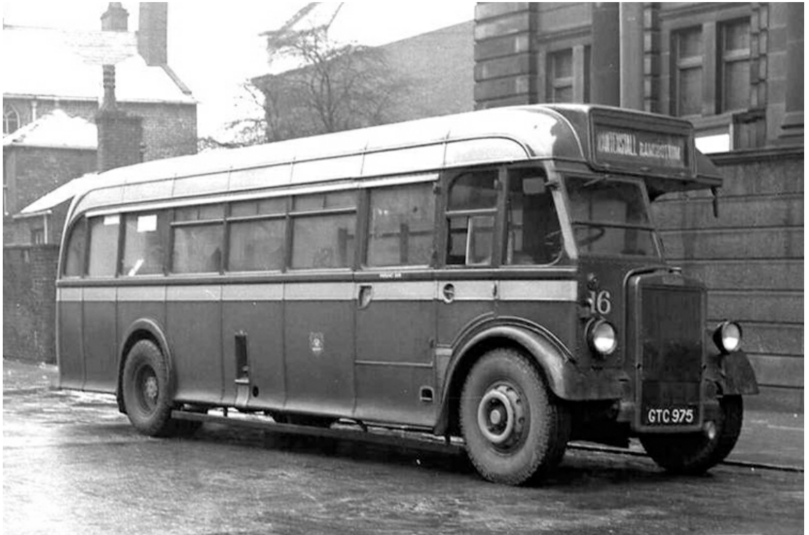
No. 16 (GTC975) was the first Leyland PS1 to enter service in 1946. It had Roe 36-seat bodywork and is seen here outside Bury Art Gallery ready to depart on the Bury to Ramsbottom service. (John Kaye).
