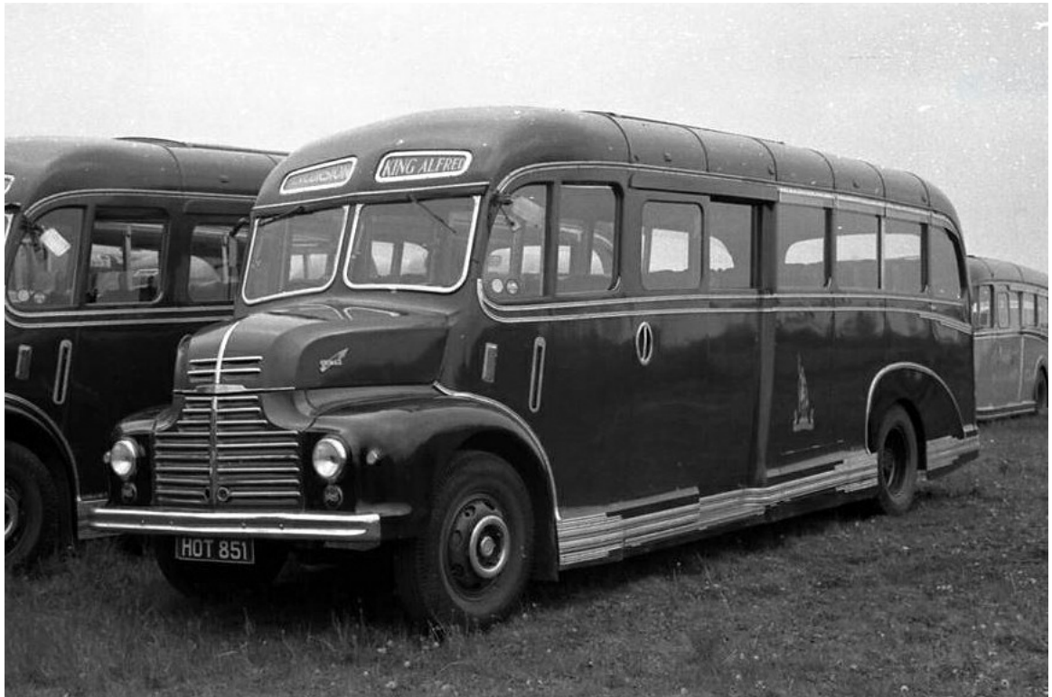
HOT851 was a 1950 Leyland Comet CPO1 in the fleet of King Alfred Motor Services of Winchester. It had Reading 33-seat coachwork and is seen here on a day trip to Whipsnade Zoo in 1959. (John Boylett courtesy John Kaye).
