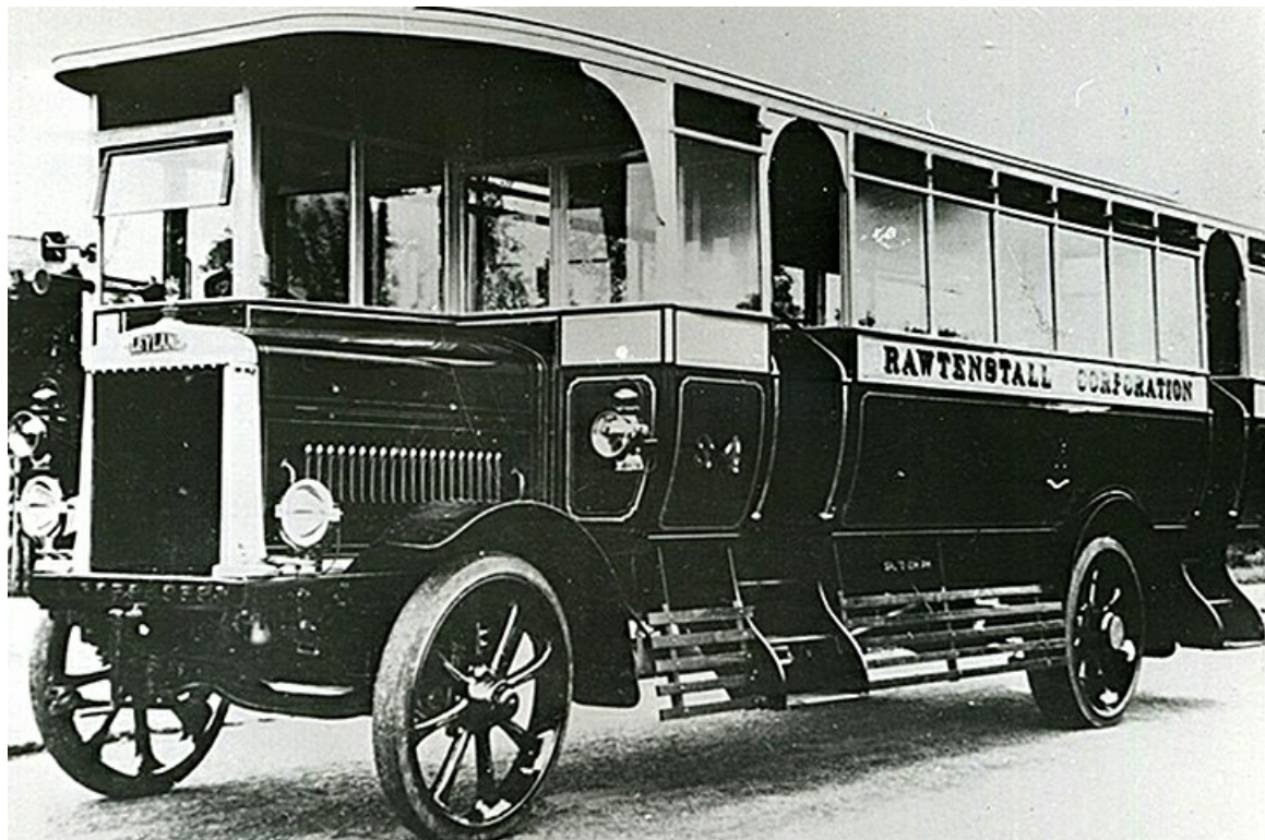
Rawtenstall Corporation No. 34 was a 1924 Leyland SG9 with Leyland 40-seat dual-entrance bodywork. (LTHL collection).
