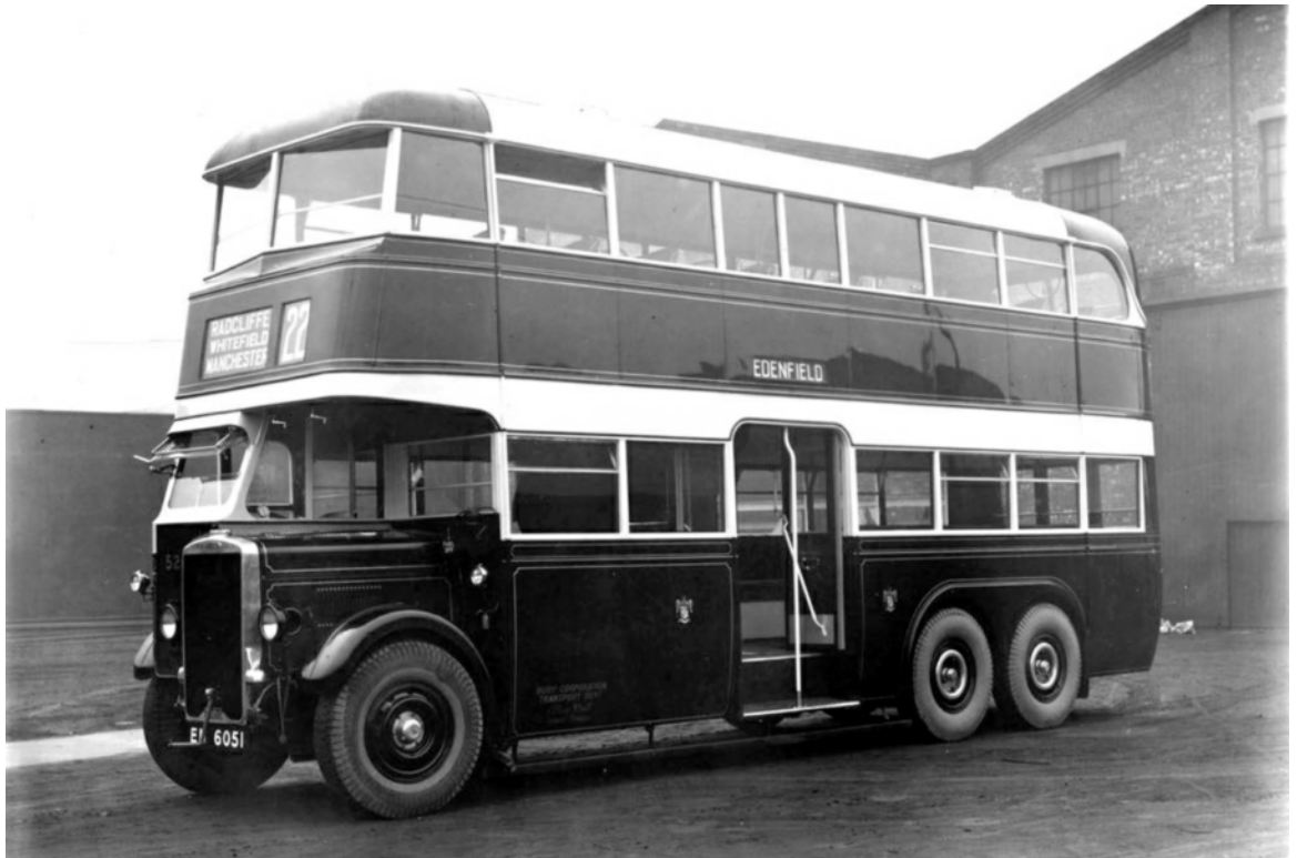
Bury Corporation ordered 5 Leyland Titanic TT3 6-wheel double-deckers in 1935 with English Electric 60-seat centre-entrance bodywork. This is No. 52 (EN6051) that remained in the fleet until 1946. (GEC Collection courtesy David Beilby).
