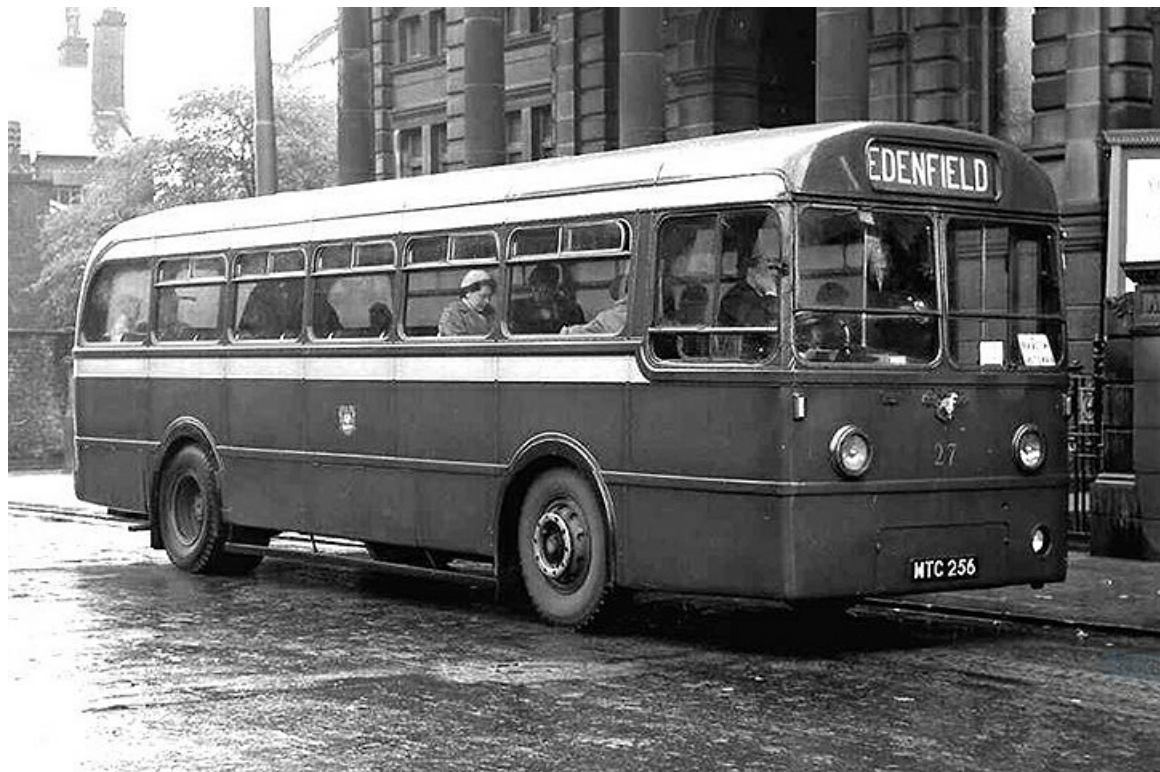
Ramsbottom No. 27 (MTC256) was a 1950 Leyland Royal Tiger, the fourth chassis built and is seen here in Moss Street, Bury in June 1958. It had a Roe 44-seat body. (John Kaye).
