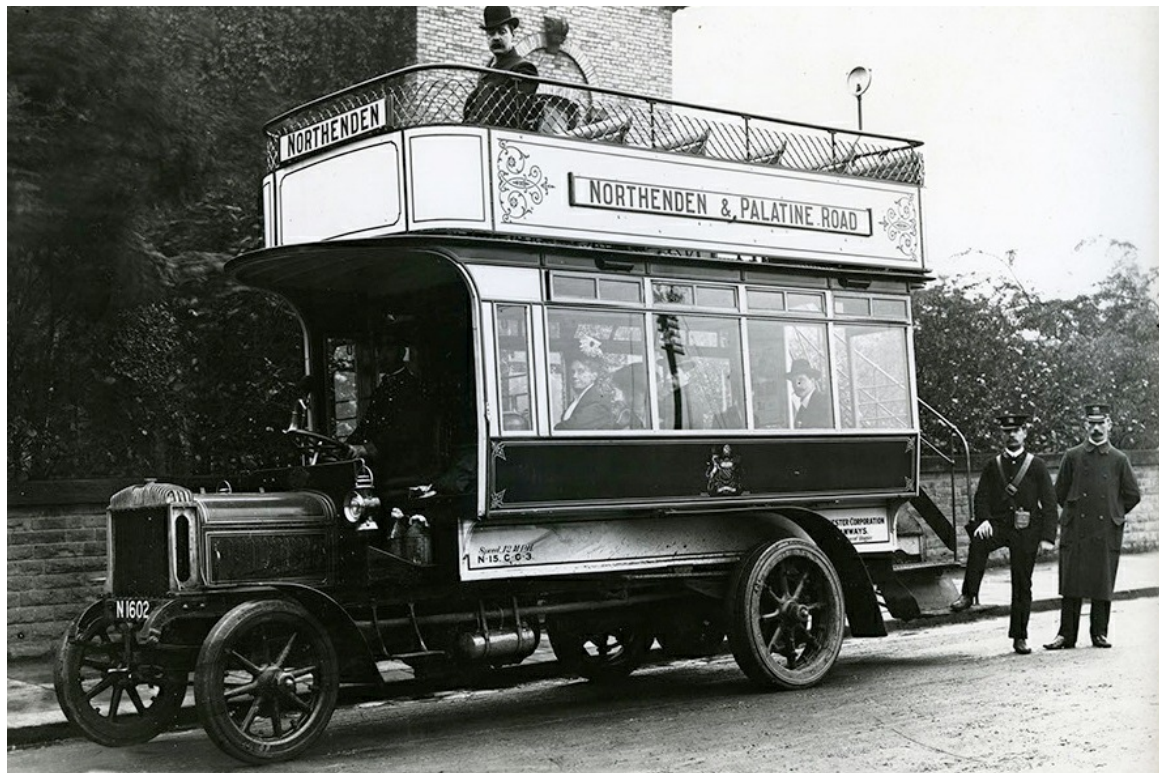
Manchester Corporation ordered this bus in 1906 from the local firm of Crossley Brothers, although the chassis were obtained from the Lancashire Steam Motor Company (the predecessor of Leyland Motors) and bodied by Dick Kerr of Preston. (LTHL collection).
