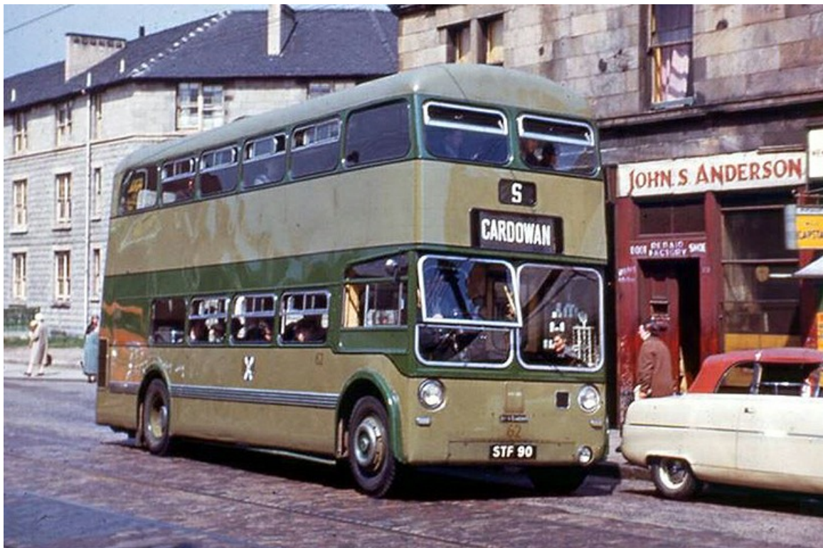
STF90 was a Leyland Lowloader, the second prototype of the Leyland Atlantean, new in June 1954. Although it had a rear engine it was constructed with a rear entrance Saunders-Roe body. It is seen here in service with Lowland Motorways of Glasgow. (John Boylett collection courtesy John Kaye).
