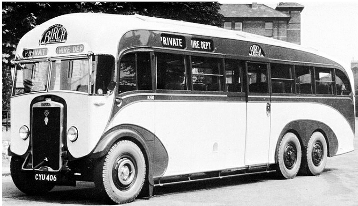
K50 (CYU406) was a 1936 Leyland TS7T (the 'T' suffix meaning trailing axle) with Birch Brothers 43-seat full front coachwork. It was re-bodied by Birch in 1943 as a 64-seat double-decker and re-numbered K150 and withdrawn in this form in 1951. (LTHL collection).
