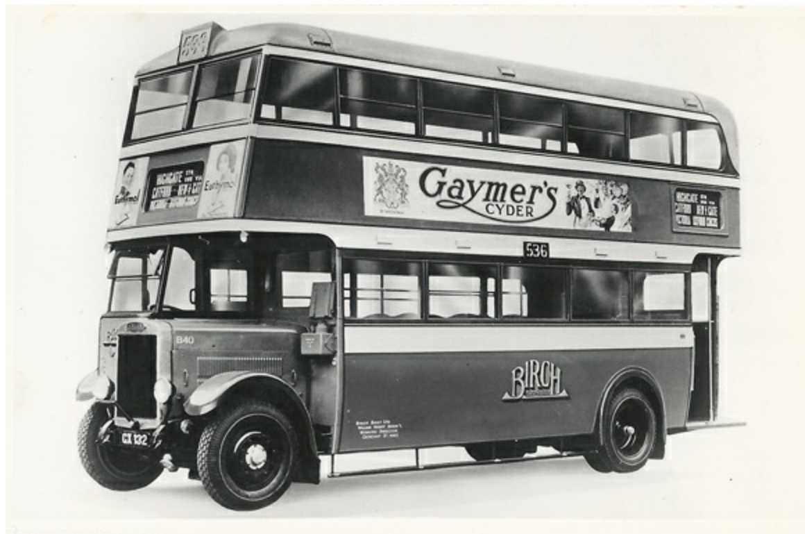
B40 (GX132), a 1932 Leyland TD2 with Birch Brothers 56-seat bodywork. It also passed to London Transport in 1934 where it became TD84. (courtesy Brian Townsend).
