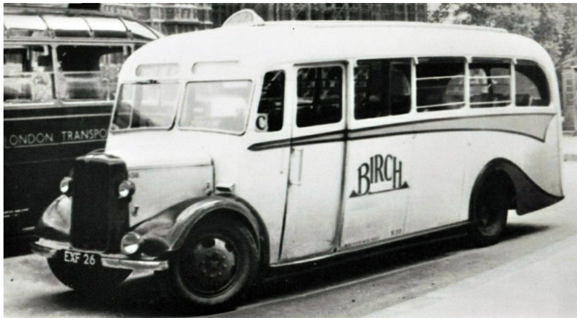
K58 (EXF26), a 1938 Bedford WTB with Birch 25-seat coachwork. It remained in service until 1949. (LTHL collection).
