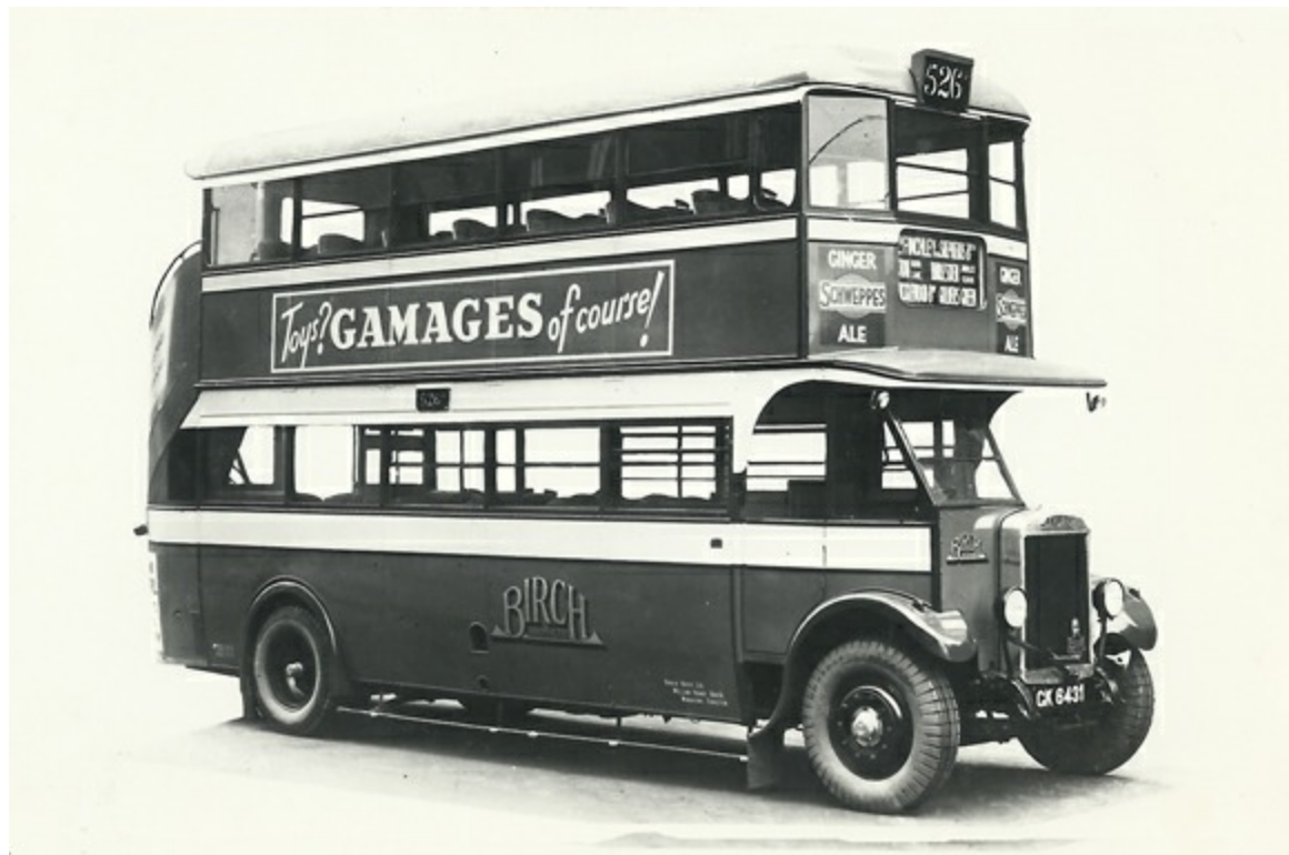
B29 (GK6431), a 1930 Leyland TD1 with Birch Brothers 56-seat bodywork. It passed to London Transport in 1934 where it became TD74. (courtesy Brian Townsend).
