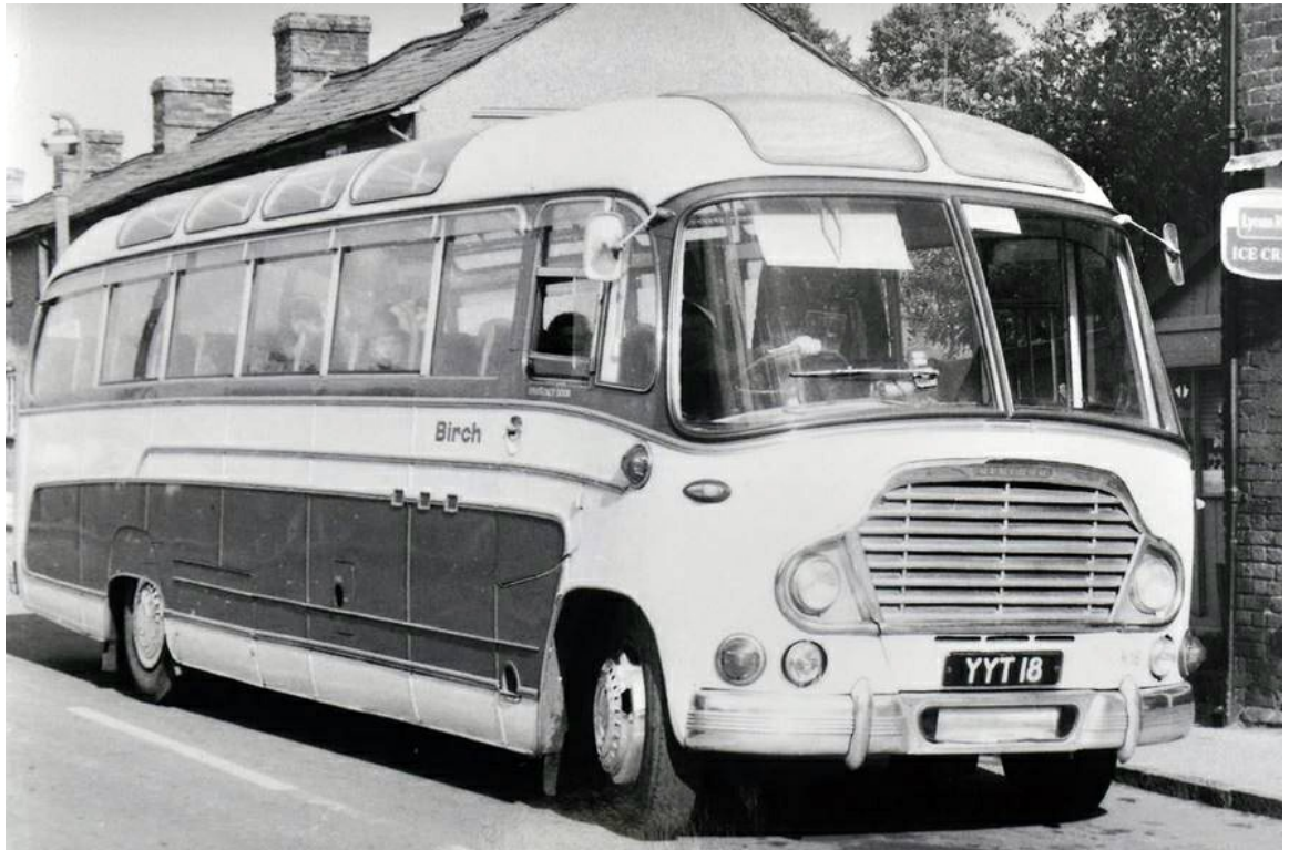
K18 (YYT18), a 1960 Bedford SB1 with Duple 41-seat bodywork - one of six similar vehicles entering service that year. All were withdrawn in 1969. (LTHL collection).
