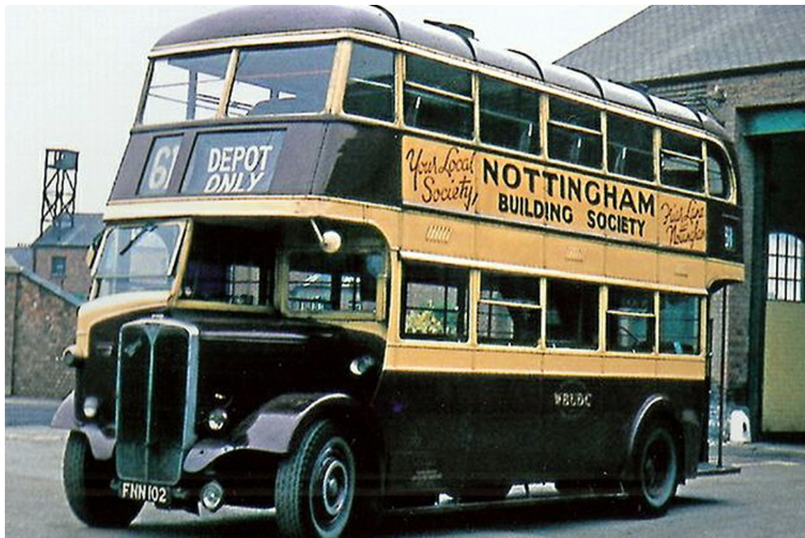
No. 4 (FNN102) was a 1939 AEC Regent originally with Park Royal highbridge 56-seat bodywork, but seen here after it was rebuilt by Willowbrook with a lowbridge 52-seat body in 1953. (LTHL collection).
