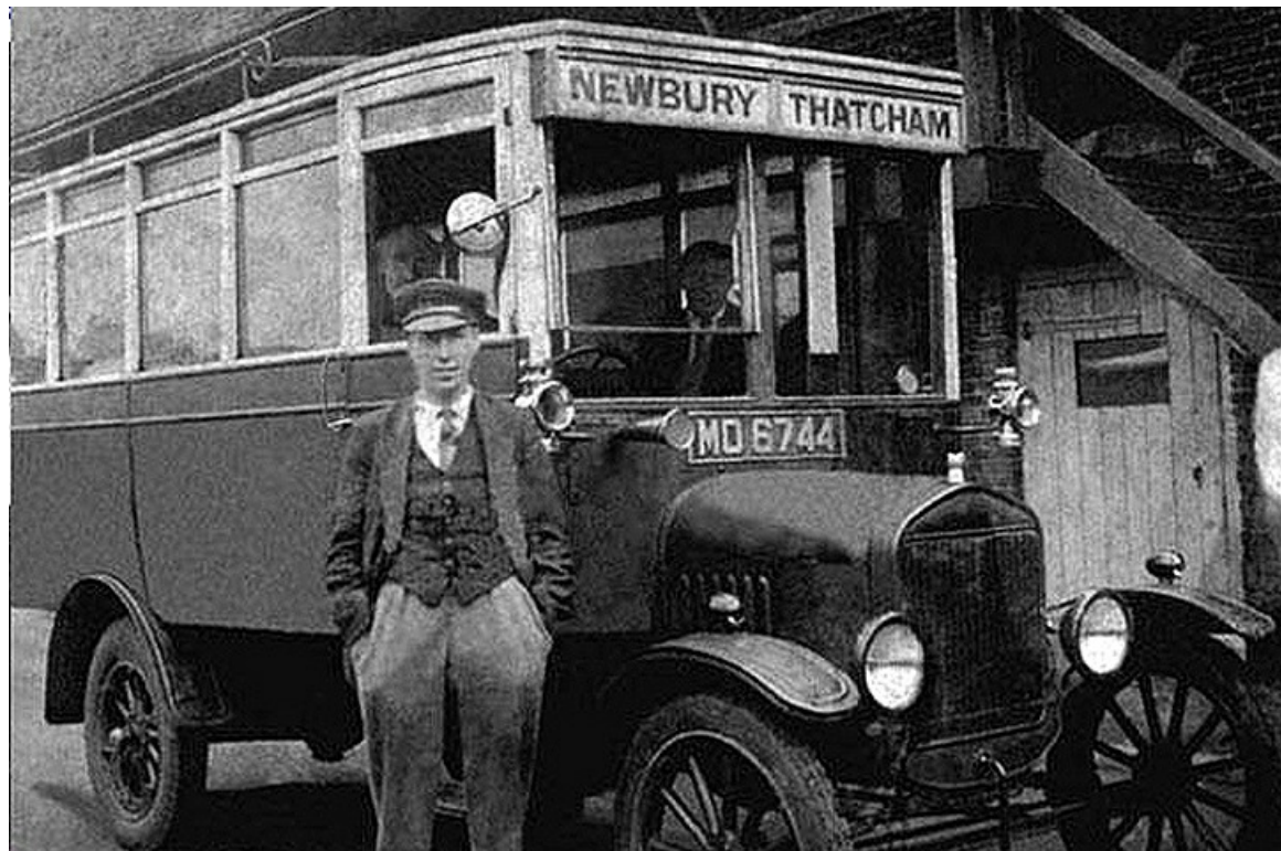
Acquired with the business of Spanswick's Bus Services in 1933 was this 1926 Ford TT with Andrews 14-seat bodywork. It was withdrawn after only a few months. (LTHL collection).
