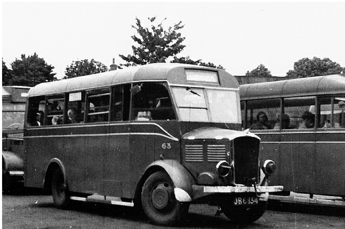
No. 63 (JB6834) was the first new vehicle purchased by Newbury & District and was also the first of many Dennis Aces acquired from 1935 onwards. It carried a King & Taylor 20-seat coach body. (The Bus Archive).
