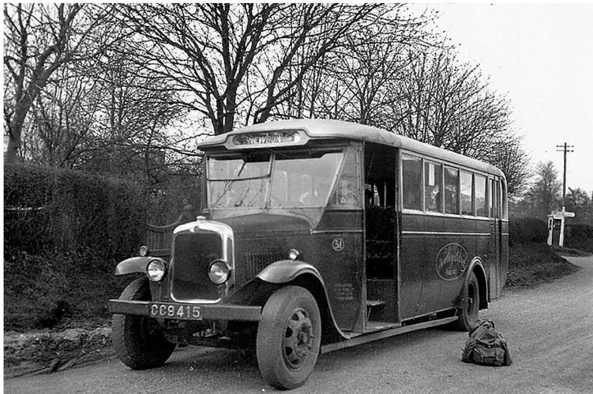
No. 31 (CC9415) was a GMC T60 with Strachan 26-seat dual entrance/exit bodywork, new in 1930 to the Tocia Motor Omnibus Company and came via Crosville Motor Services in 1934, when Tocia were acquired. (The Bus Archive).
