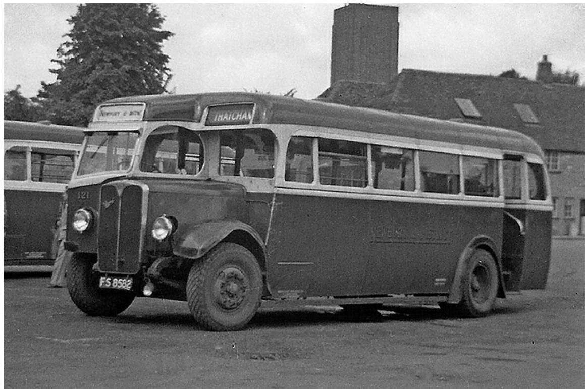
No. 121 (FS8582) was an AEC Regal 4 that had been new in 1934 and was acquired from the War Department in a run down state, completely rebuilt and re-bodied with an ex-North Western Road Car ECOC/ECW body. (The Bus Archive).
