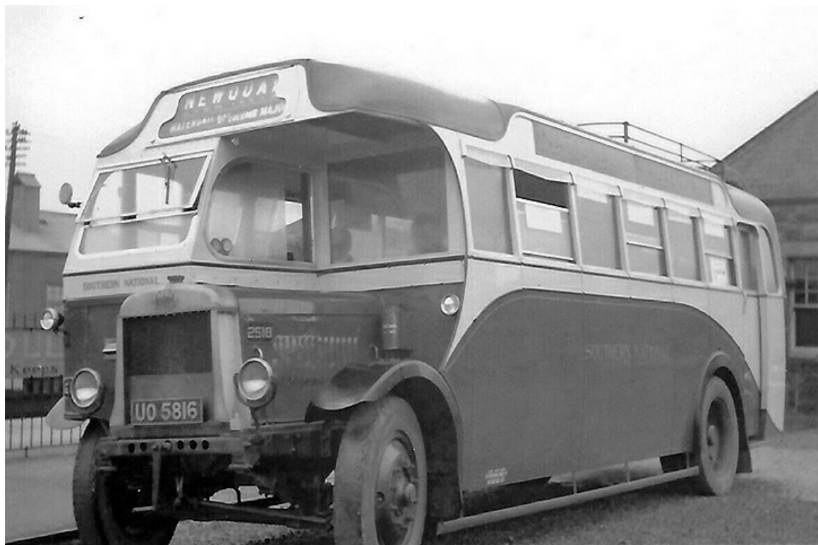
No. 2518 (U05816) was a 1928 Leyland LSC3 inherited from the National Omnibus & Transport fleet. It originally carried Strachan & Brown B32R bodywork, but is seen here with the later 1937 Mumford B32R body. (Bus Archive).
