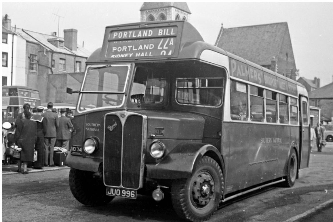
No. 1074 (JU0996) was an AEC Regal III dating from 1948 with Strachans B35R bodywork. (Bus Archive).
