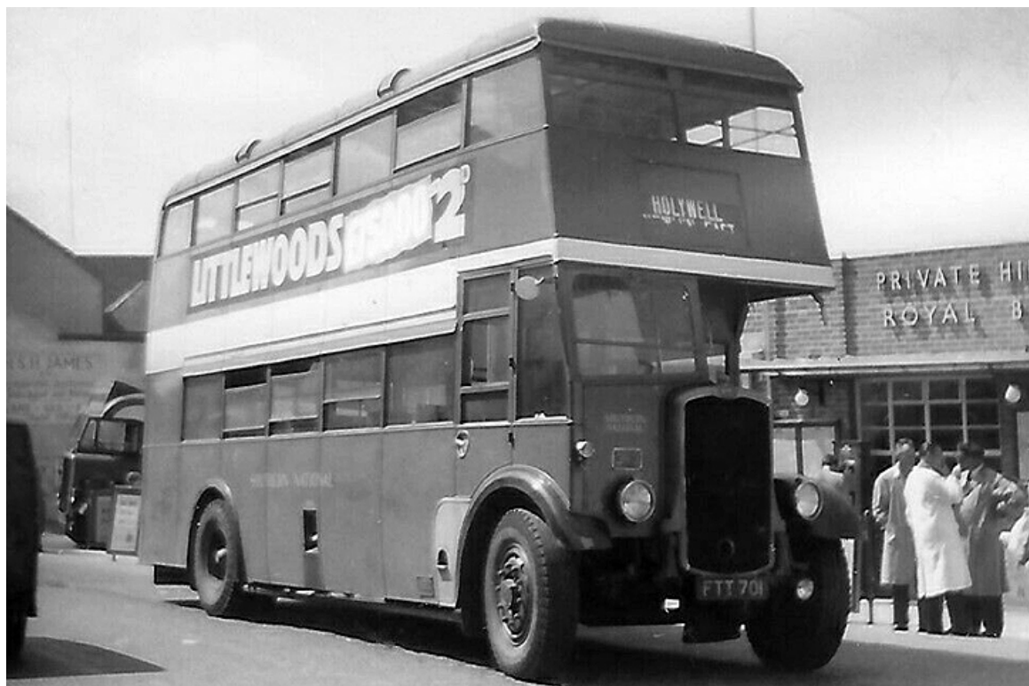
No. 363 (FTT701) was a 1945 Bristol K6A with Strachans utility L27/28R bodywork. (LTHL collection).
