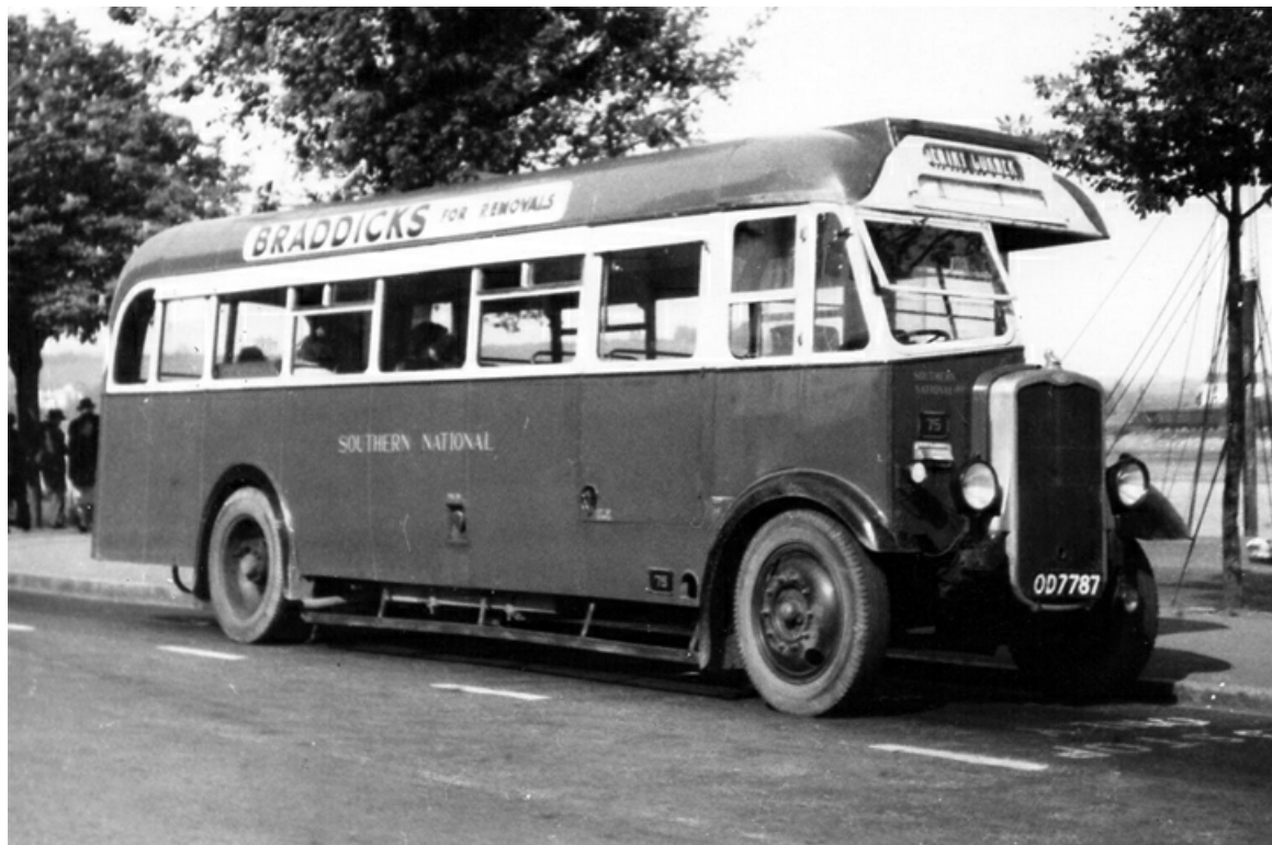
No. 75 was another TSM B39A7 dating from 1934 but seen here in 1950 with a Beadle B35R body and Bristol PV2 radiator. (LTHL collection).
