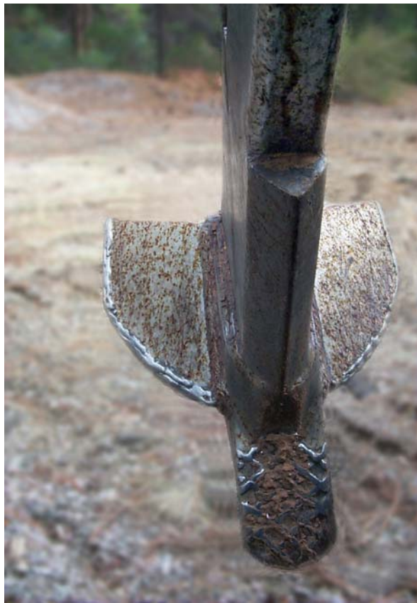
Figure 10.1.2.2. Soil shattering becomes more effective when wings are mounted on subsoil tines. This equipment is called a winged subsoiler. Photo courtesy Brent Roath.
