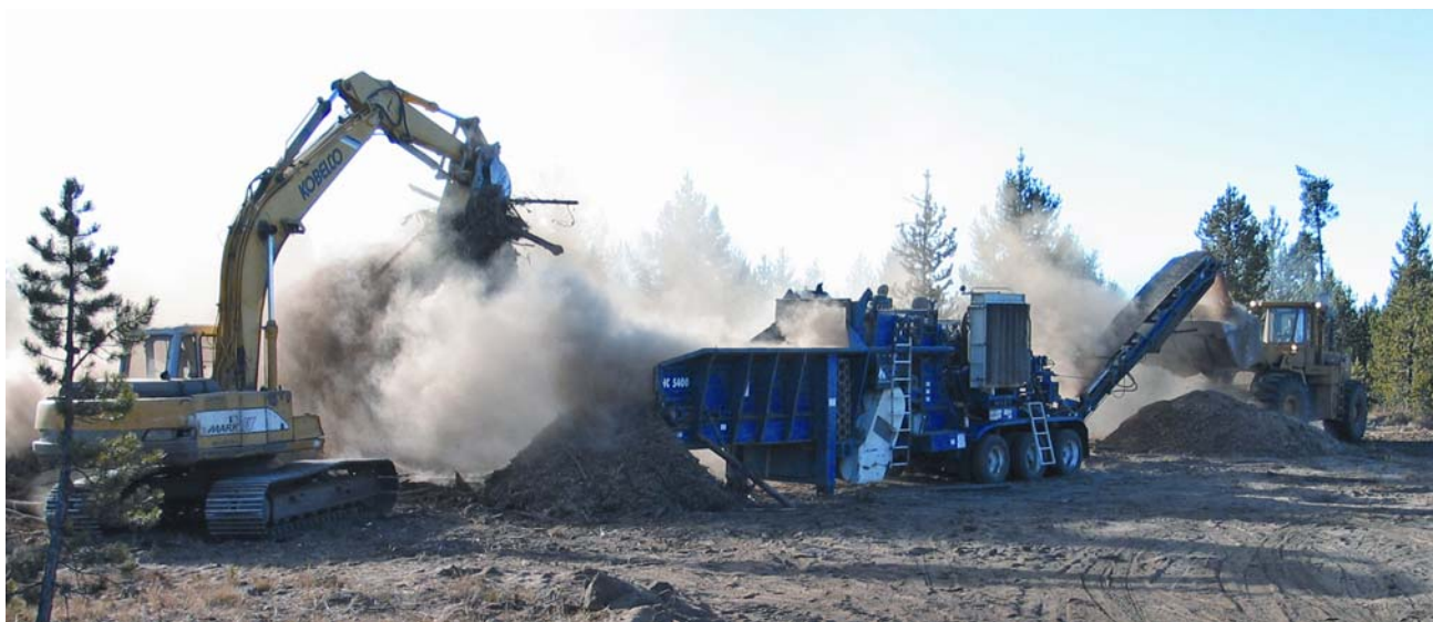
Figure 10.1.3.7. Large mulching operations require access and working space. The operation shown in this photograph shows the wood waste material being dropped into a grinder with an excavator (left), and conveyed as mulch to the bucket of a front end loader (right).
