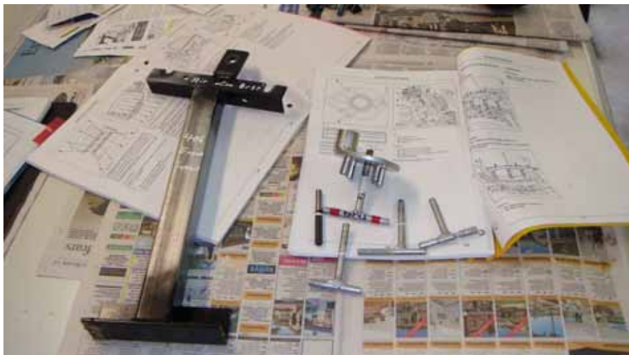
A picture of the tools you need to make. I used a worn socket welded to the cam tool.
