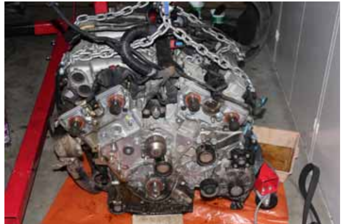
Another V6 engine (not Steve's) that shows the rear timing covers and all cam gear removed.
