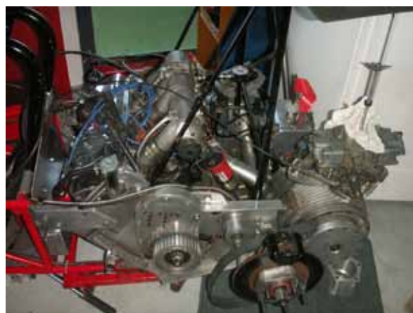
Kiwi dragster: A well-worked over 1967 Peugeot 404 engine with Ti head, Holley double pumps and a 50lb boost home-made supercharger has powered this flyer to an 8.9 second quarter mile and made V8 guys cry. It was a highlight of an Auckland club display in 2008.
