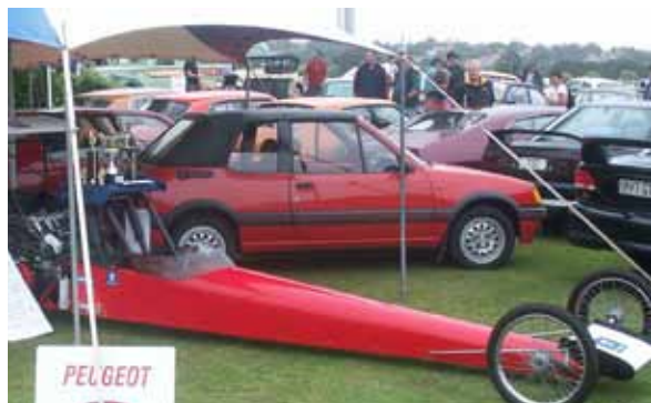
Kiwi dragster: A well-worked over 1967 Peugeot 404 engine with Ti head, Holley double pumps and a 50lb boost home-made supercharger has powered this flyer to an 8.9 second quarter mile and made V8 guys cry. It was a highlight of an Auckland club display in 2008.
