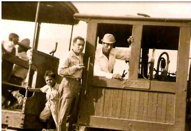
A US-built saddle tank, possibly the same as in the previous photo, bearing the name 'STA. MARÍA'.
