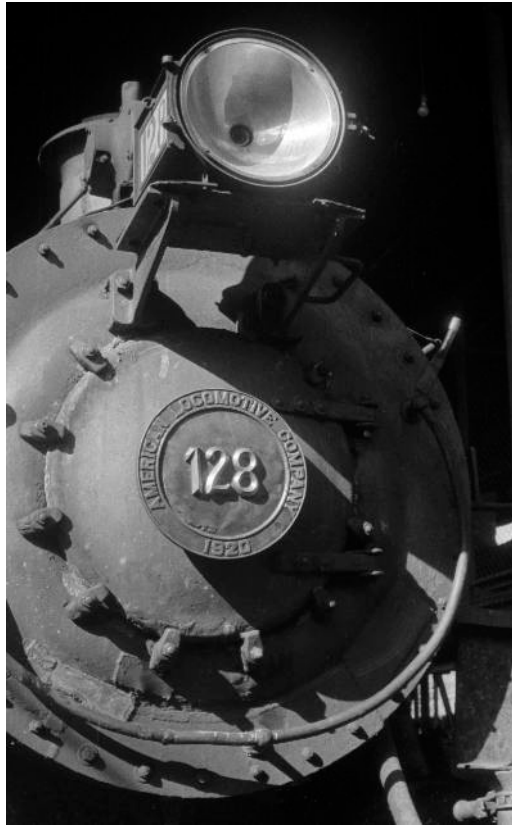
No. 128 's front number-plate, presumably the original background and peripheral lettering saying 'AMERICAN LOCOMOTIVE COMPANY', but having had the central numbers changed at least twice.
