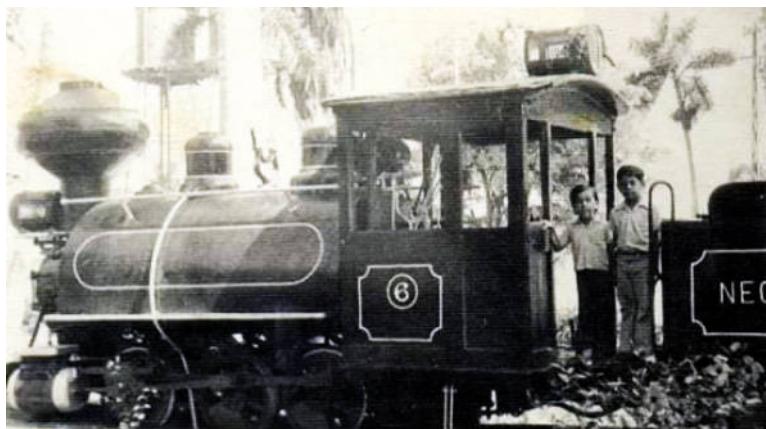
Hacienda Tumán no. 6, seemingly retro-fitted with a Rushton stack, and possibly with a name beginning 'NEG...' on the tender.
