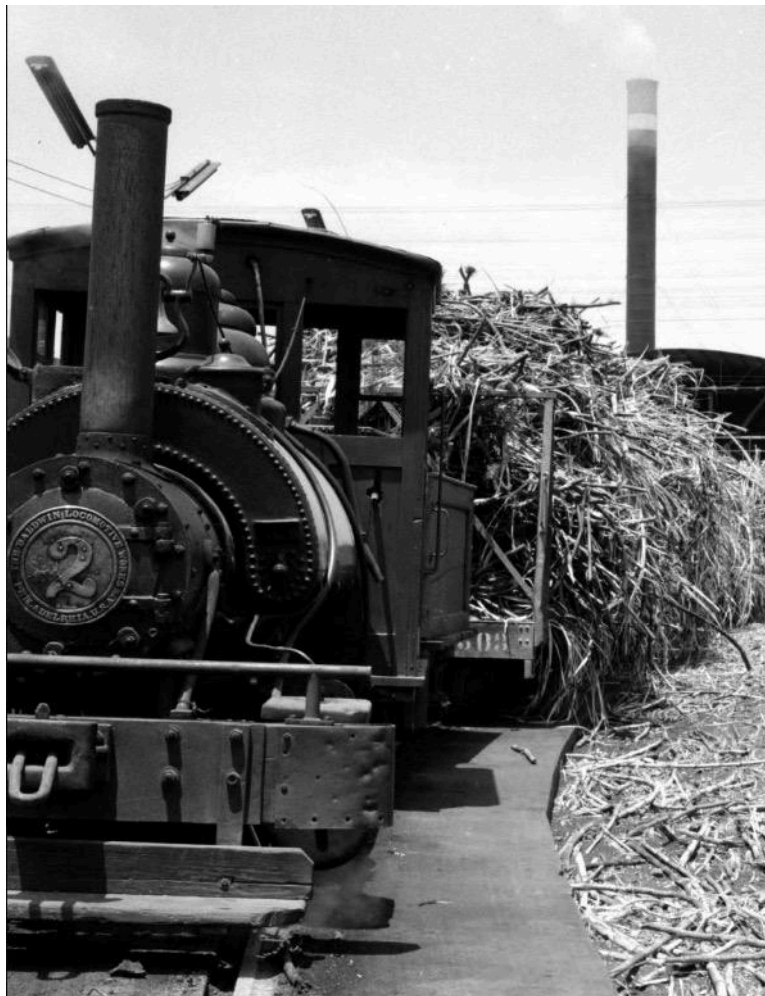
This photo of no. 2 was taken in the late 1950s or early '60s if the striplights cantilevered from poles behind the engine are any guide. It also looks as though a tender has been attached to the loco, and the loss of the original Radley & Hunter stack might mean that oil was now the fuel. The steam dome also seems considerably lower, so maybe the loco had been reboilered.
