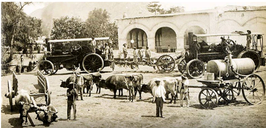
A pair of Fowler ploughing engines at Hacienda San Nicolas, together with the appropriate balanced plough.
