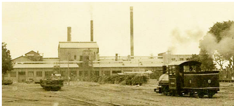
This cropped view of the Hacienda Pomalca yard shows loco no. 6 to have been an American-built 0-6-0STT with a name on its cabside.
