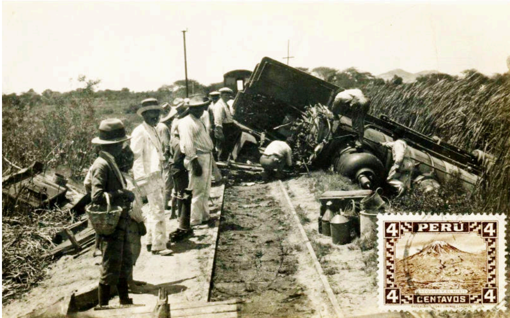
A serious derailment to an American-built loco on what would appear to be a 3' 0", metre or 3' 6" gauge railway, possibly around 1930. The engine has its dome over the firebox, implying an older design, and the boiler length and visible connecting rod suggest that it might have been a 2-6-0 or 4-4-0. This image appears on the Facebook page Antiguas Fotos de Chiclayo as having occurred on the railway between Chiclayo and the Hacienda Pátapo possibly in the 1950s.
