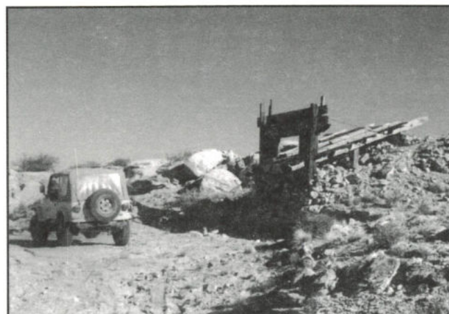
Ore loading chute at Yellow Cat Mesa Mine. Mine openings and core holes are above the chute.
