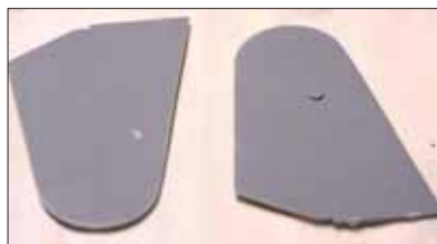
Above: Two of the horizontal tail components reveal some of the fit problems encountered throughout the kit. The ejection pins have to be removed, the mating surfaces evened and the edges dressed before the parts can be glued.
