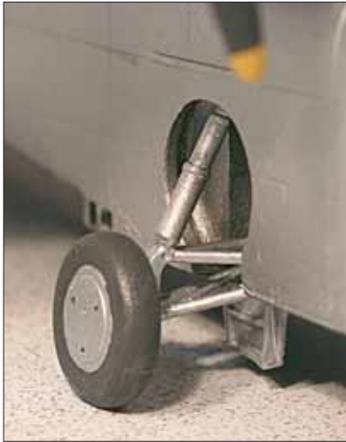
A good view of the completed main landing gear showing the three-armed assembly at the lower joint and the two-armed assembly at the upper joint.
