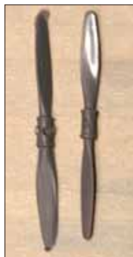
Left: Czech Model's propellers can be used as a basis, but the flash will have to be removed, the edges thinned and the blades filled where the injection-moulded plastic is incomplete. There is also a problem with the propeller hubs, which are inaccurate. The modeller will either have to scratch build new propeller hubs, or cover them with the spinners.
