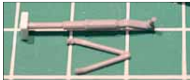
Above: The main gear strut was cut to remove excess length. By slowly and carefully fitting the parts inside the gear well, the length was adjusted through the square fitting made at the top. This was achieved by cutting off small lengths of excess until everything was even.
