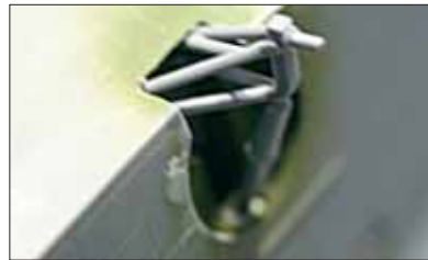
Above: The main gear is glued together, adding both the upper and lower struts. After cleaning up and resizing all the fittings, liquid glue was used to attach all the components. After the glue had dried, another coat was applied and it was left to dry again over a period of a couple of days. The result was an adequately strong joint, although the plastic itself is not very resilient and the wheel attachment arm was replaced with metal rod.
