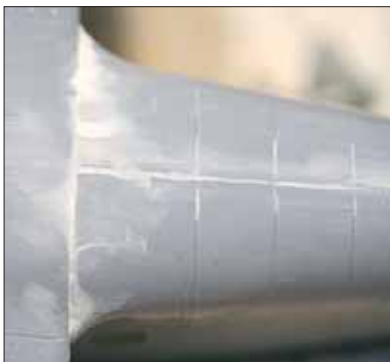
Above: Ordinarily, David compensates for a poor fit by attaching the components from top to bottom or from front to back. In this case, the fit was so bad that he elected to fit the wing from back to front. A great deal of cutting, sawing, filling and sanding were needed to get a good fit. Once the wing had been fitted correctly, the panel lines had to be rescribed.
