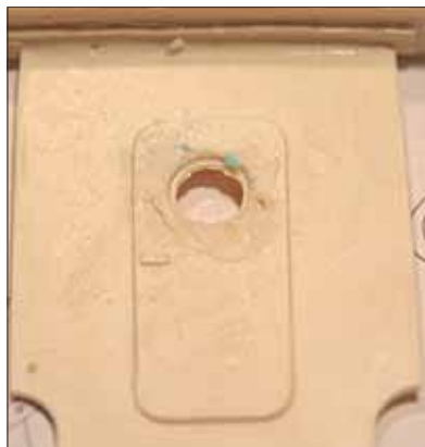
Above: In addition to the problems with the injection-moulded plastic, there were also missing and malformed resin parts on David's model. The interior cabin door was incompletely moulded and required cleaning up and rebuilding.
