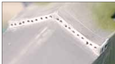
Above: The hull drainage component to be glued under the hull step was inaccurate. A new item was therefore fabricated using scrap 20-thou plastic.
