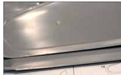
Above: The upper and lower wing halves had very thick edges, which required sanding on a flat surface to ensure a true mating surface for gluing. Considerable time was spent thinning the trailing edges with a knife before sanding smooth.
