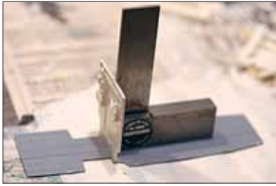
Above: Whenever parts assembly required the application of a right angle, David used a steel square as a jig to ensure that the angle was correct as the glue dried.
