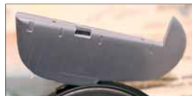
Above: Having glued the two rudder halves together, the process of cleaning out the hinge locations and adding the pivot arm can begin.
