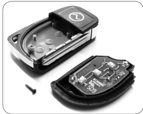
1. Remove screw on the back of the key fob and open the housing.
