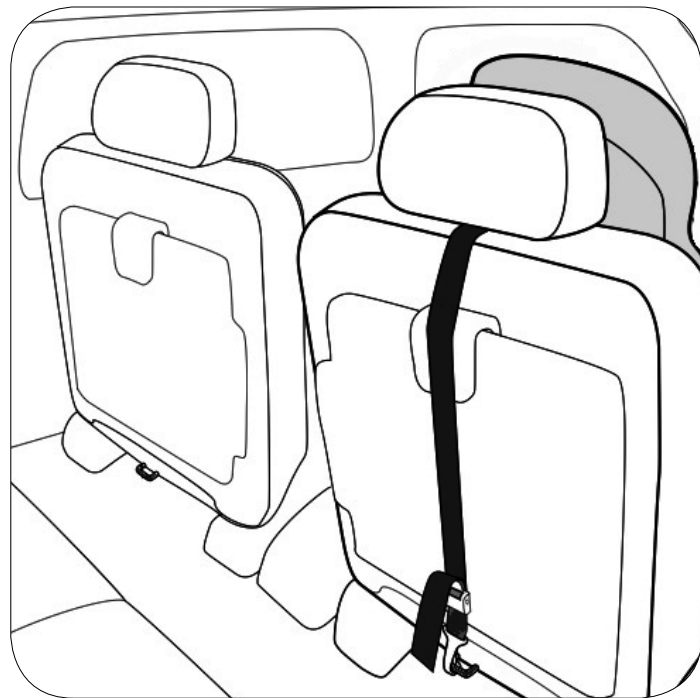
2. Raise the head rest, put the strap(s) under it, then attach to the rear anchor point on the lower back side of the seat.
