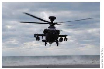
AH-64E modified with Spike NLOS missile hovers off the coast of Florida before engaging overwater target at 32km.
