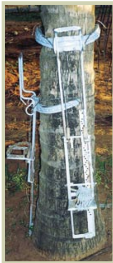
Figure 6-3. A simple and effective two-piece climbing frame invented in India, which enables anyone of moderate strength to gain access to the crown of a coconut palm.
