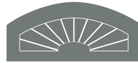
EYEBROW WITH LEGS Square sides, with a slight radius to a full radius top. Side louvers have almost full rotation.
