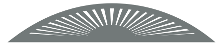
ELONGATED EYEBROW ARCH Rotation of louvers is limited on both ends, but offers almost full rotation of the louvers in the center.
