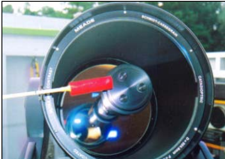
Figure 3. Possible position of the Homebrew Collimation Tool between two set screws to indicate that it is the opposite single screw that is to be adjusted.
