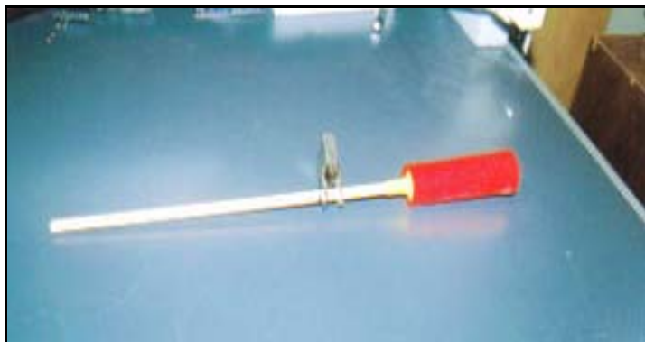
Figure 1. The Homebrew SCT Collimation Tool by Bill Black.
