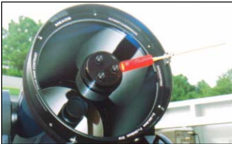
Figure 2. Position of the Homebrew Collimation Tool to indicate which collimation screw to adjust.
