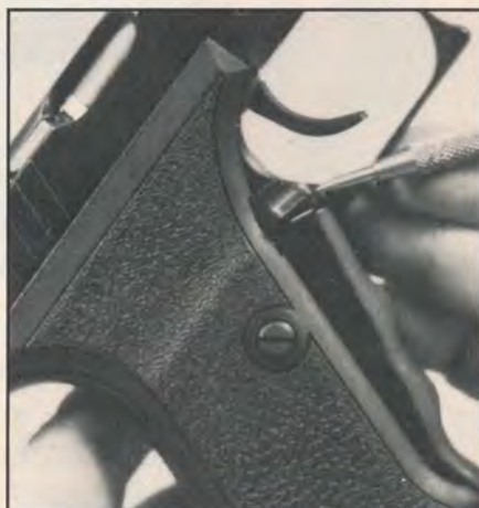
The author points to the port side of the ambidextrous magazine release button, which is pushed downward to release.
