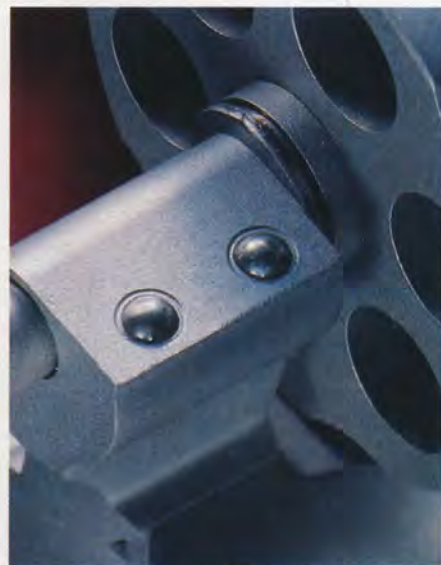
The crane is locked to the frame with not one but two ball detent locks. Weigand says this aids in better accuracy, and obviously it's stronger.
